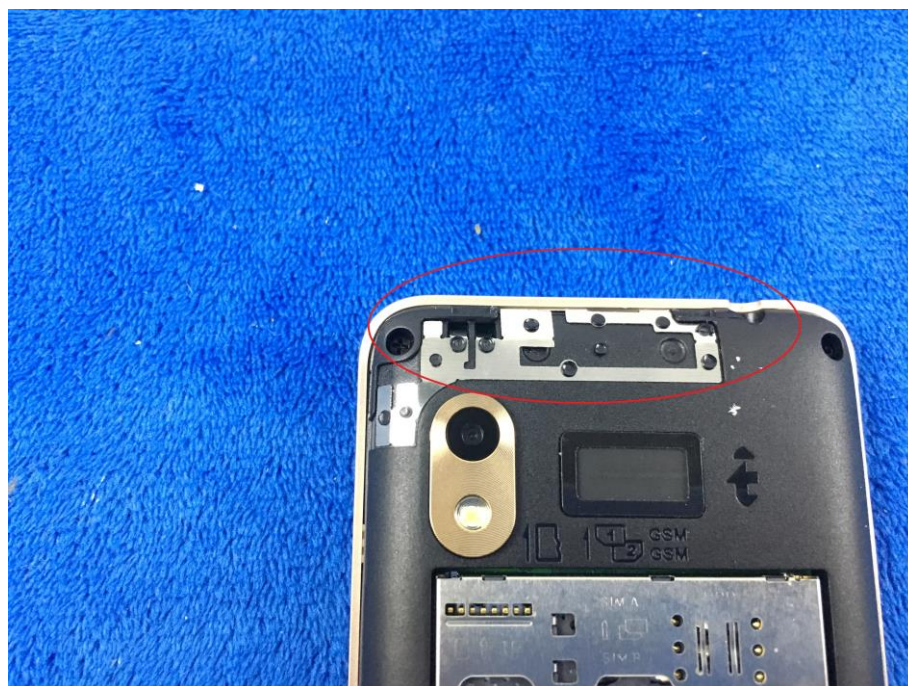
GSM/PCS/UMTS-FDD - Antenna View
