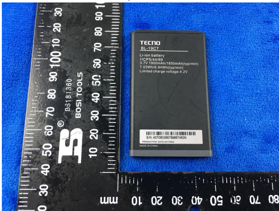
Battery - Front View
