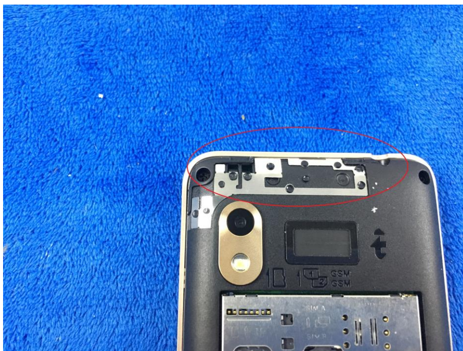
GSM/PCS/UMTS-FDD - Antenna View
