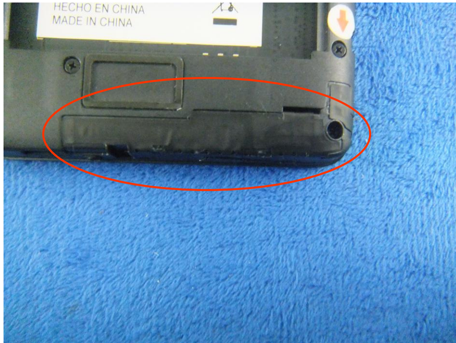
GSM/PCS/UMTS - Antenna View
