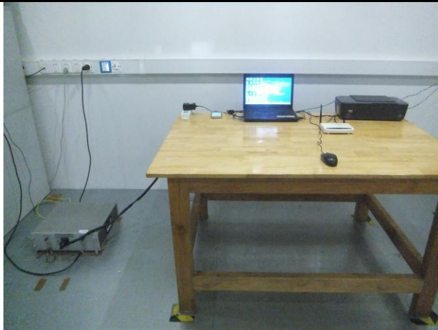
Conducted Emissions Test Setup – Front View
