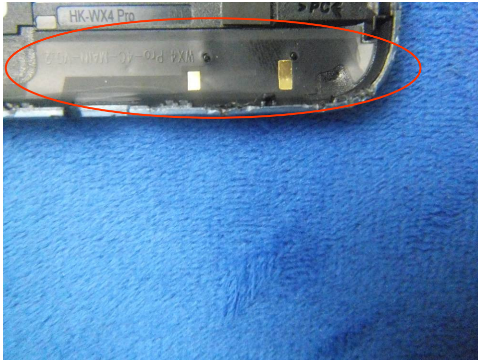
GSM/PCS/UMTS-FDD Antenna View
