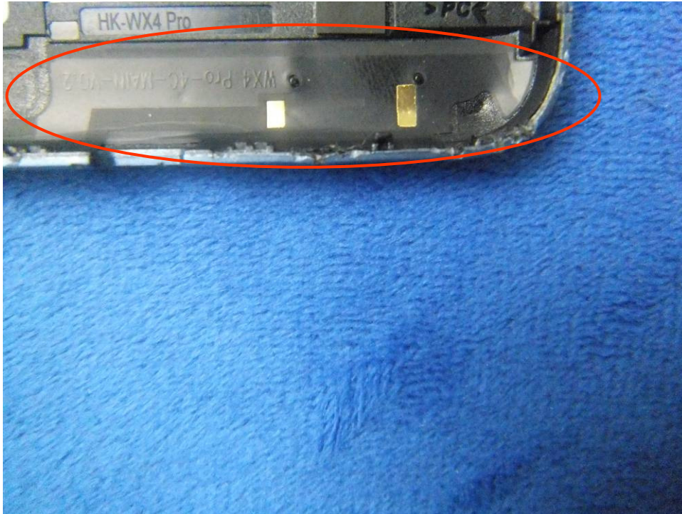
GSM/PCS/UMTS-FDD Antenna View
