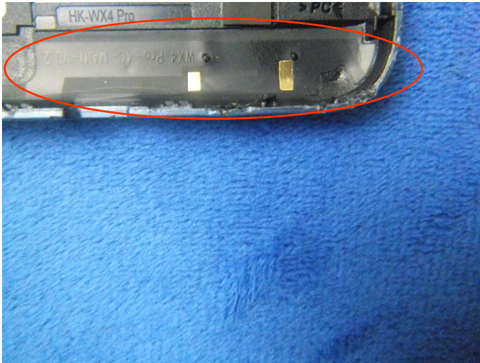
GSM/PCS/UMTS-FDD Antenna View
