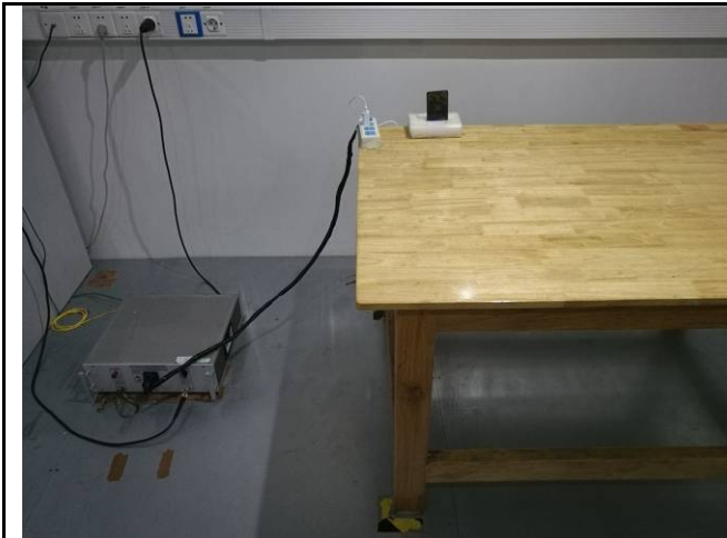
Conducted Emissions Test Setup Front View
