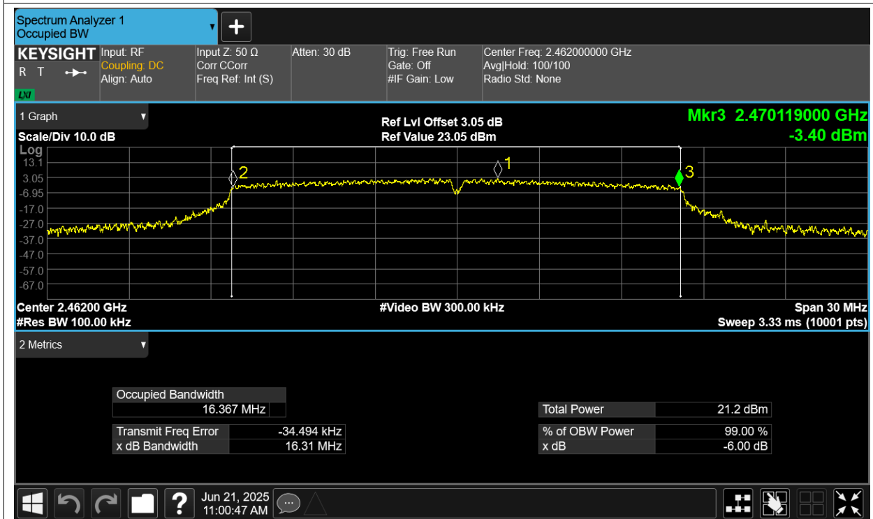
-6dB Bandwidth NVNT n20 2412MHz Ant13
