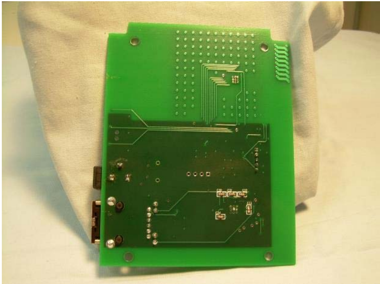
Photograph 20 – View of the Bottom Side of the HUB001 PCB
