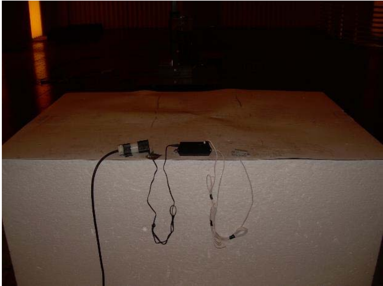
Photograph 6 – Back View of the DS001 Radiated Emission Worst-Case Test Setup
