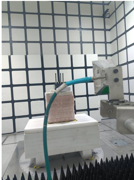
Radiated Emissions View (18-25 GHz)
