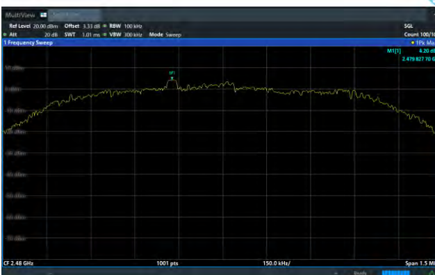
8DPSK on Channel 78
