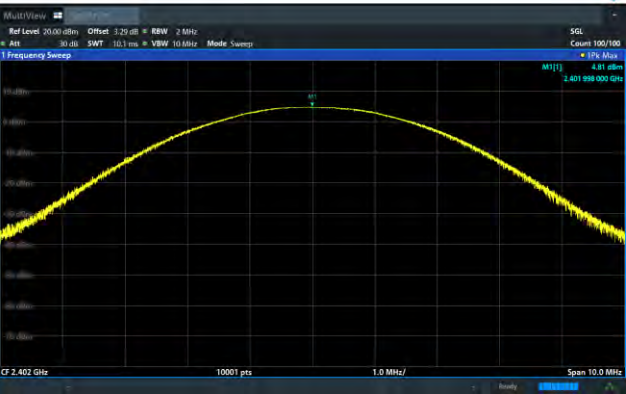
8DPSK on Channel 78
