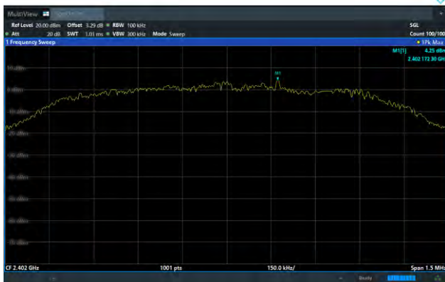
8DPSK on Channel 39
