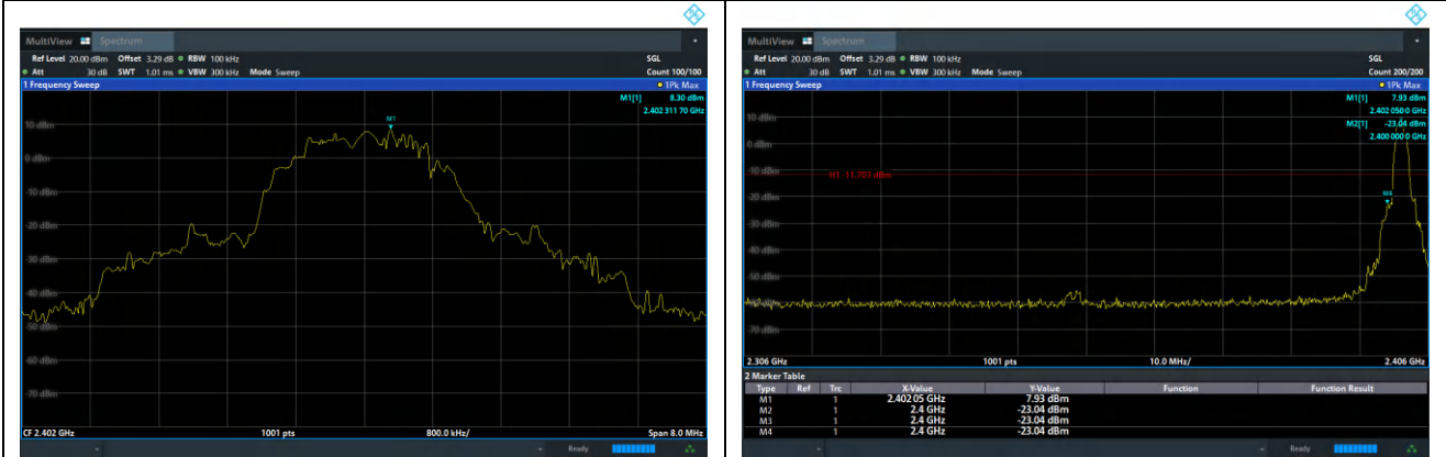
GFSK(2M): Band Edge, Right Side
