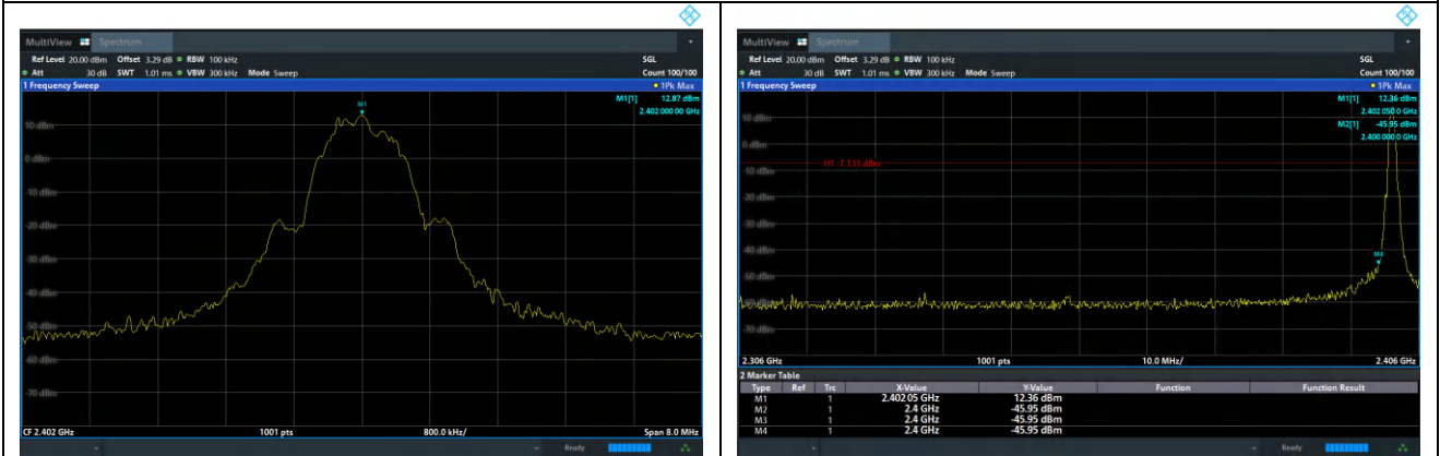
GFSK(1M): Band Edge, Right Side
