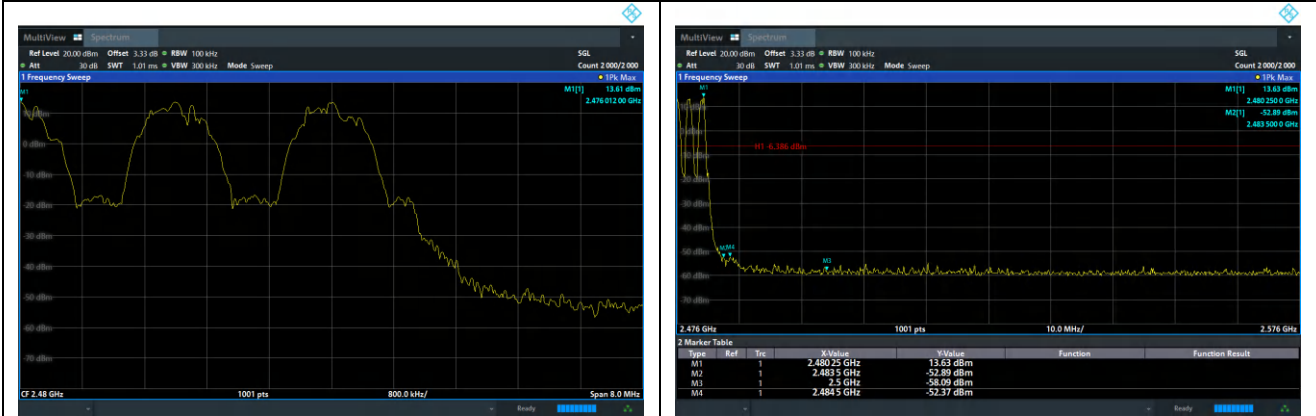
GFSK(1M): Band Edge, Right Side
