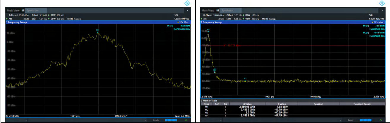
GFSK(2M): Band Edge, Right Side
