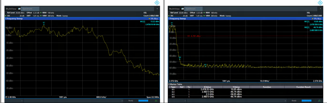
GFSK(2M): Band Edge, Right Side
