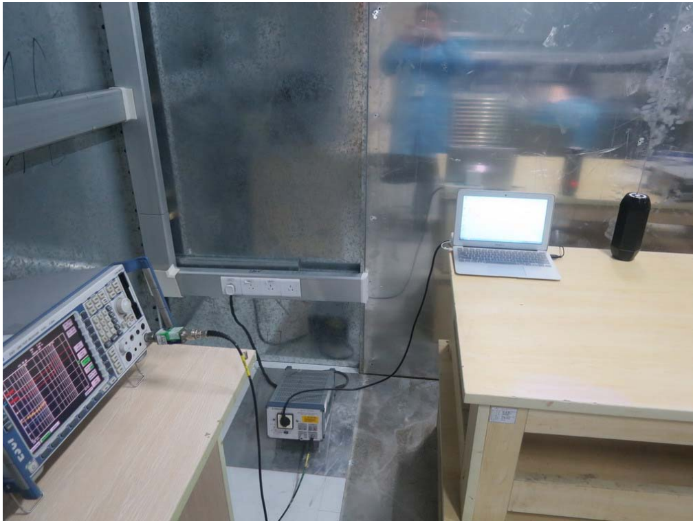
FCC RADIATED EMISSION TEST SETUP
