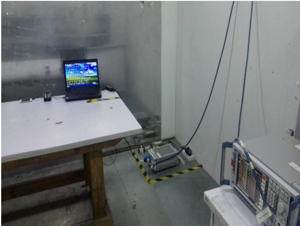
FCC RADIATED EMISSION TEST SETUP
