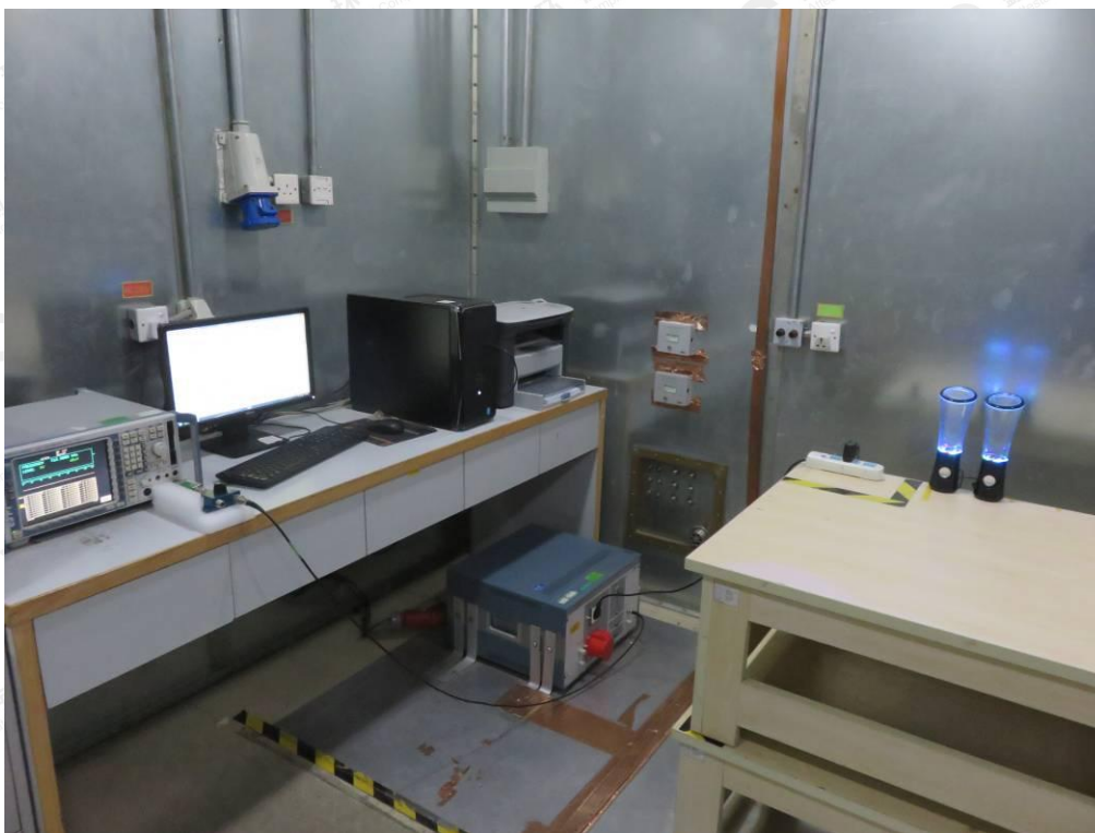
FCC RADIATED EMISSION TEST SETUP
