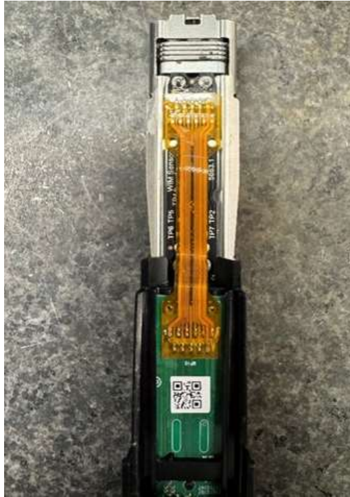
Figure 12: The flex PCB carries the NFC antenna traces from PCB1 to PCB2
