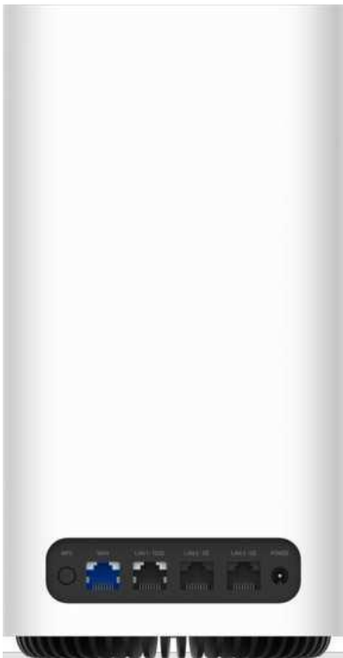
Figure 5-2 Beacon 19 physical connections
