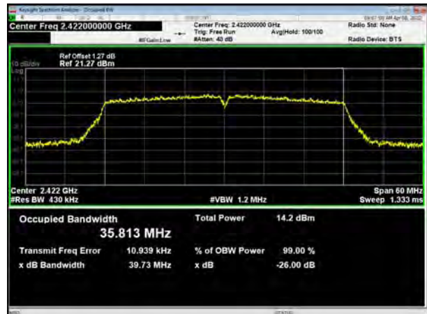
802.11n(HT40), Carrier frequency (MHz): 2437
