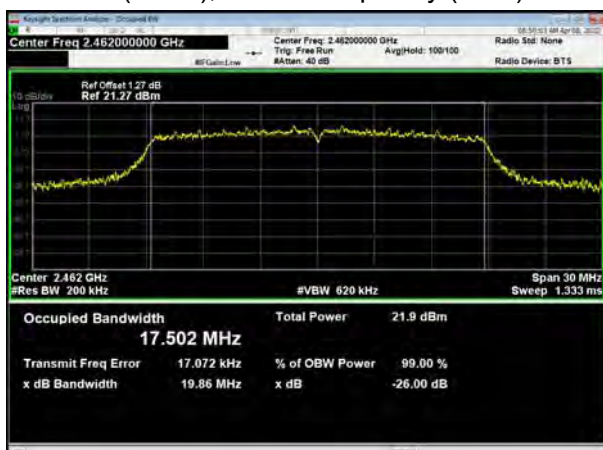
802.11n(HT20), Carrier frequency (MHz): 2462
