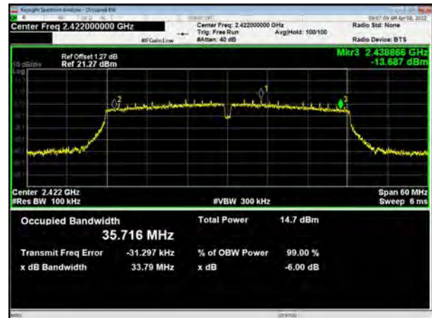
802.11n(HT40), Carrier frequency (MHz): 2437
