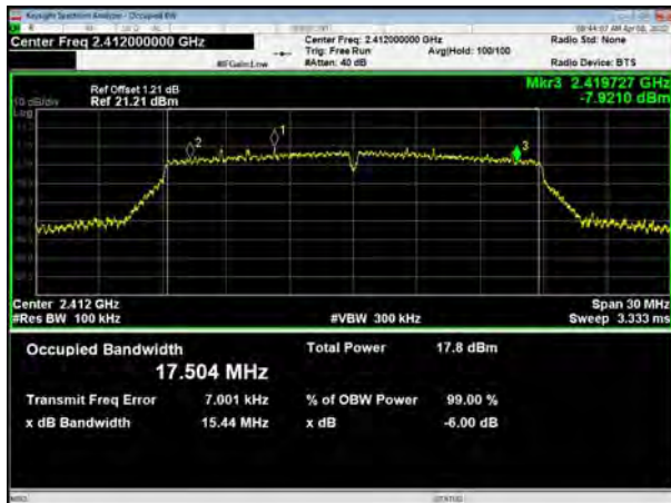
802.11n(HT20), Carrier frequency (MHz): 2437
