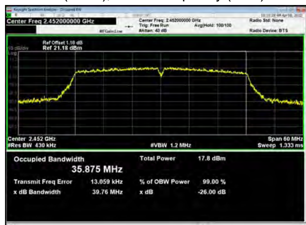
802.11n(HT40), Carrier frequency (MHz): 2452
