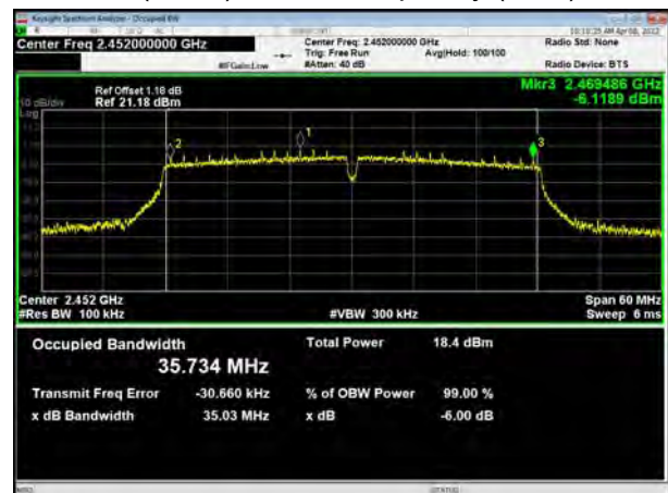
802.11n(HT40), Carrier frequency (MHz): 2452
