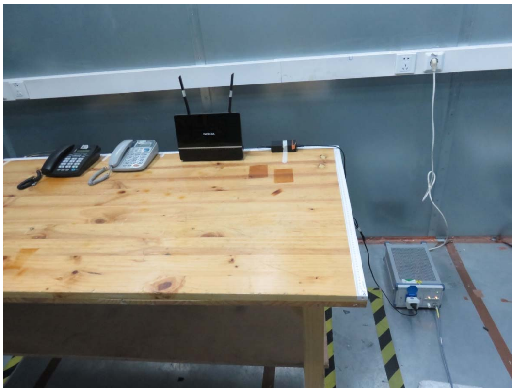
Picture 3 Conducted Emission Test Setup
