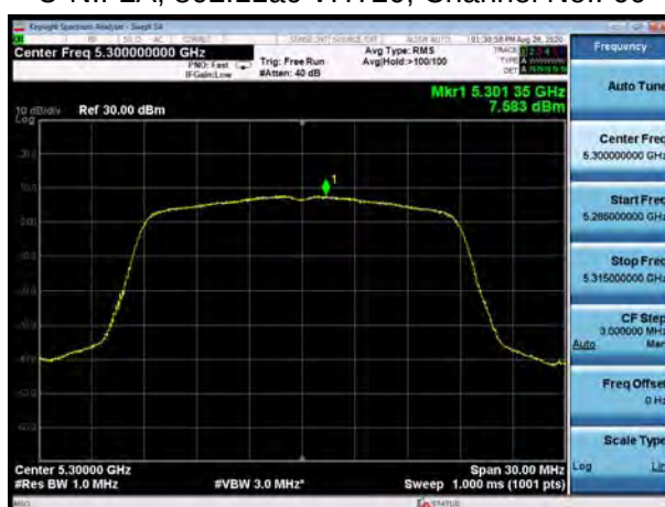
U-NII-2A, 802.11ac VHT20, Channel No.: 64
