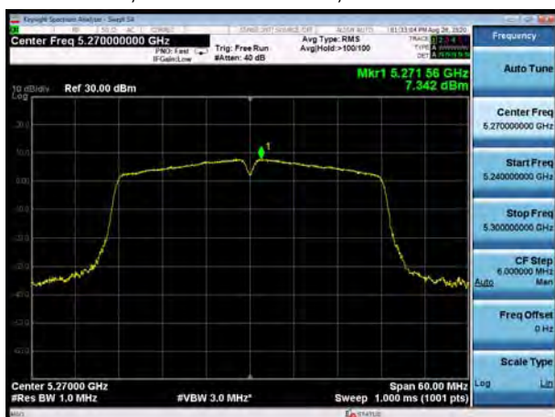
U-NII-2A, 802.11ac VHT40, Channel No.: 54
