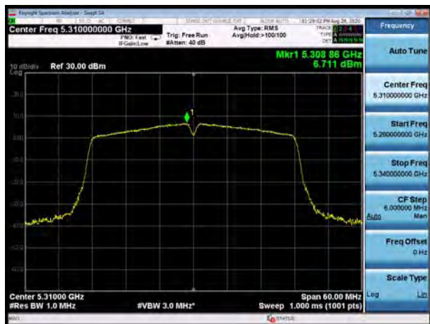
U-NII-2A, 802.11ac VHT40, Channel No.: 54
