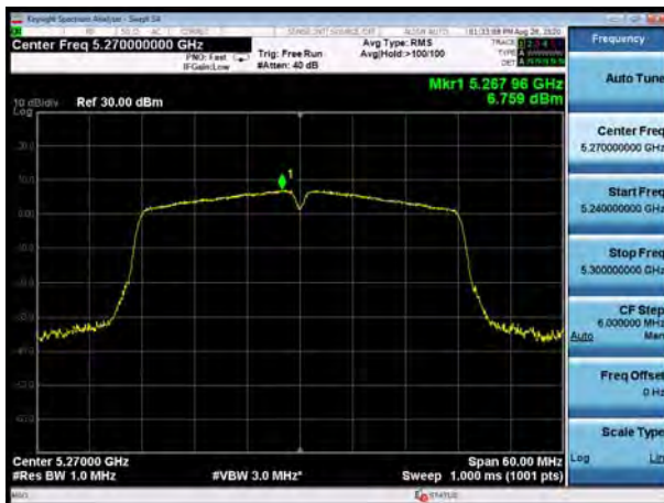
U-NII-2A, 802.11ac VHT40, Channel No.: 54
