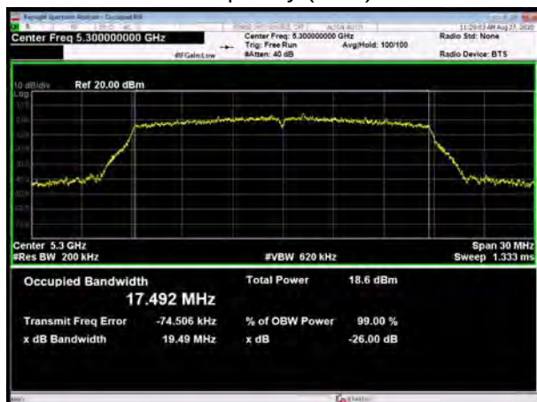
U-NII-2A, 802.11n HT20 Carrier frequency (MHz): 5320
