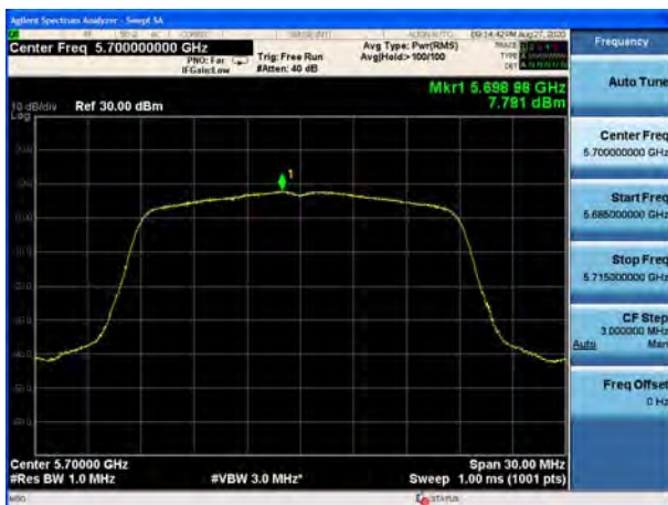
U-NII-2C, 802.11ac VHT20, Channel No.: 144
