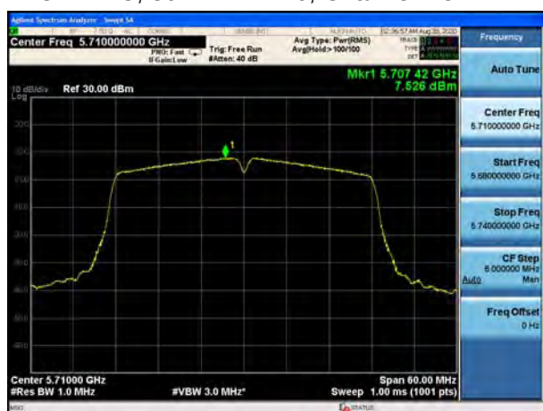
U-NII-2C, 802.11ac VHT40, Channel No.: 102
