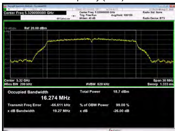
U-NII-2A, 802.11a Carrier frequency (MHz): 5320
