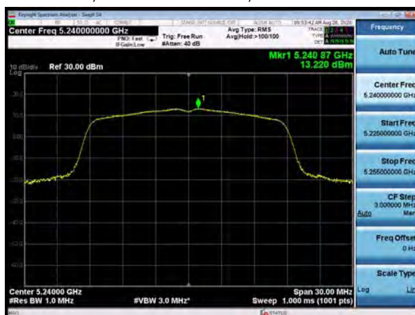
U-NII-1, 802.11ac VHT20, Channel No.: 48
