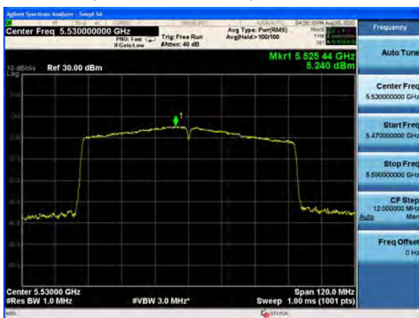
U-NII-2C, 802.11ac VHT80, Channel No.: 106
