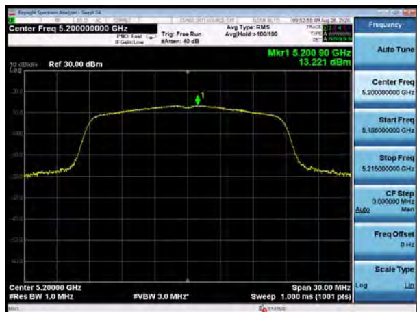
U-NII-1, 802.11ac VHT20, Channel No.: 48
