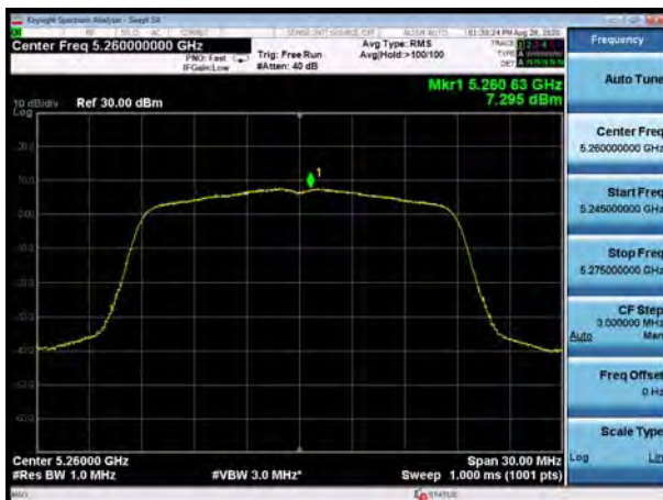
U-NII-2A, 802.11ac VHT20, Channel No.: 60
