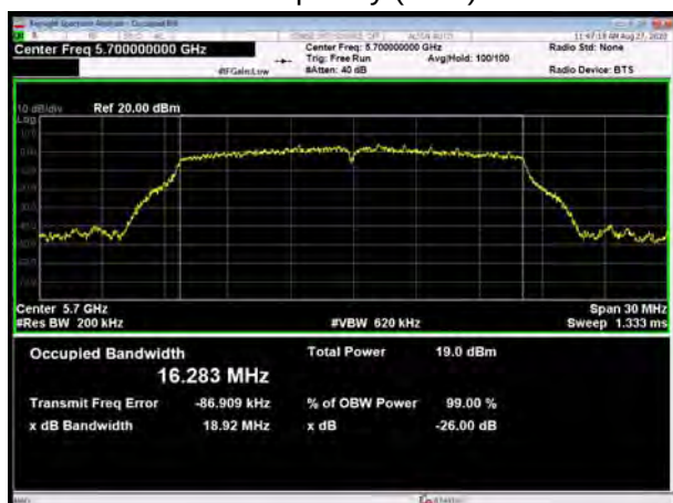
U-NII-2C, 802.11a Carrier frequency (MHz): 5700
