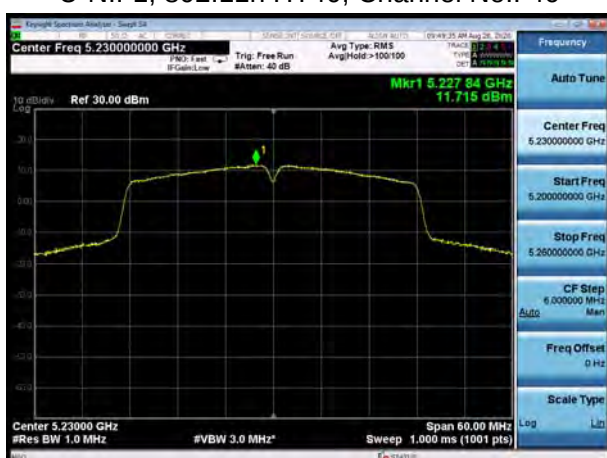
U-NII-1, 802.11ac VHT40, Channel No.: 38
