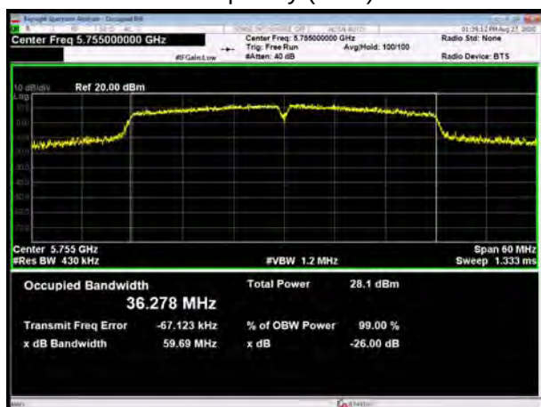
U-NII-3, 802.11n HT40 Carrier frequency (MHz): 5795
