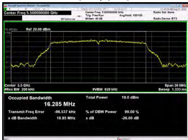
U-NII-2C, 802.11a Carrier frequency (MHz): 5580
