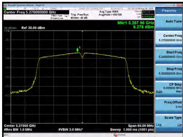
U-NII-2A, 802.11ac VHT40, Channel No.: 54
