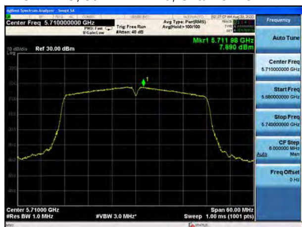
U-NII-2C, 802.11ac VHT40, Channel No.: 102
