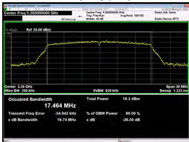
U-NII-2A, 802.11n HT20 Carrier frequency (MHz): 5300
