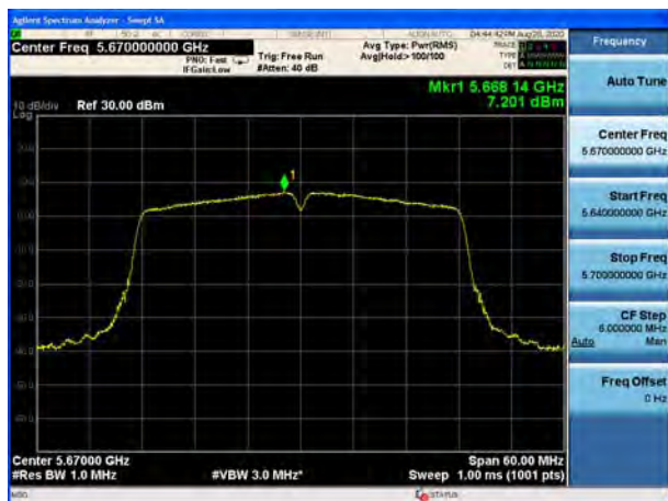
U-NII-2C, 802.11ac VHT40, Channel No.: 142
