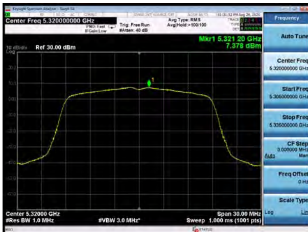
U-NII-2A, 802.11ac VHT20, Channel No.: 64
