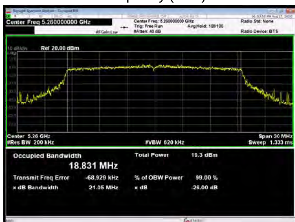
U-NII-2A, 802.11ax HE20 Carrier frequency (MHz): 5300
