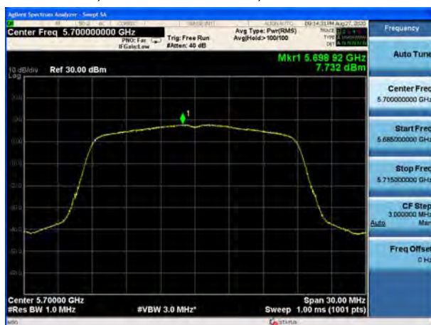
U-NII-2C, 802.11ac VHT20, Channel No.: 144
