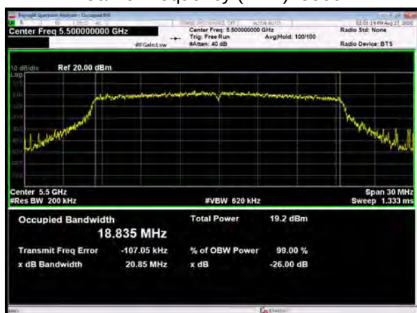
U-NII-2C, 802.11ax HE20 Carrier frequency (MHz): 5580
