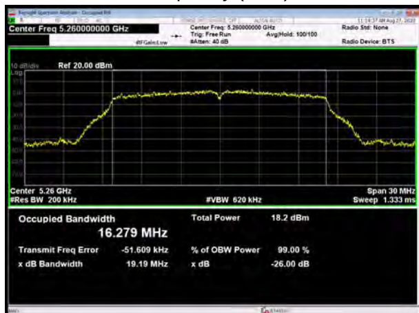
U-NII-2A, 802.11a Carrier frequency (MHz): 5300
