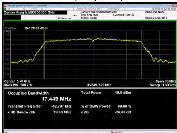
U-NII-2C, 802.11n HT20 Carrier frequency (MHz): 5700
