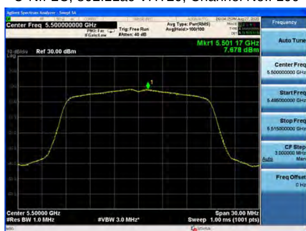
U-NII-2C, 802.11ac VHT20, Channel No.: 116
