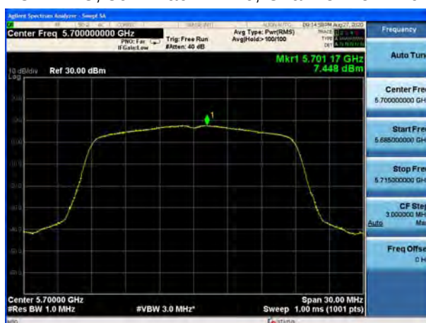
U-NII-2C, 802.11ac VHT20, Channel No.: 144
