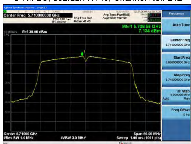
U-NII-2C, 802.11ac VHT40, Channel No.: 102
