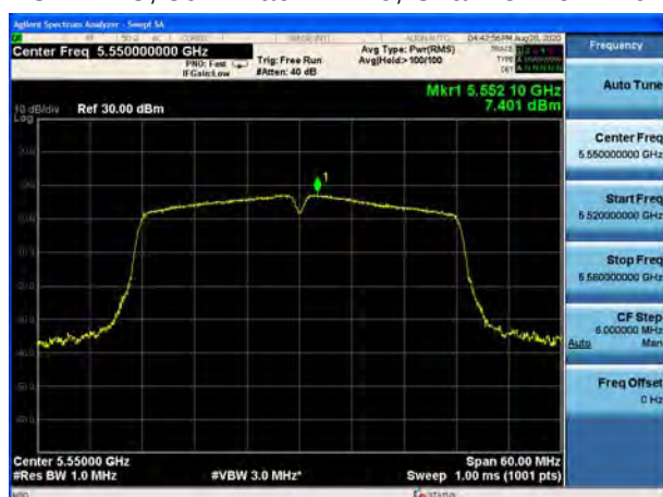
U-NII-2C, 802.11ac VHT40, Channel No.: 134
