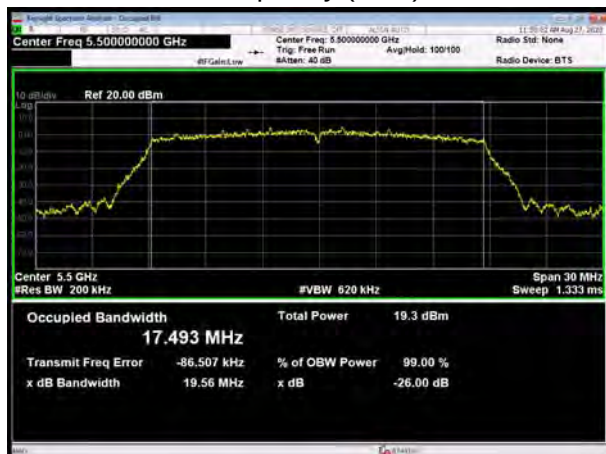
U-NII-2C, 802.11n HT20 Carrier frequency (MHz): 5580
