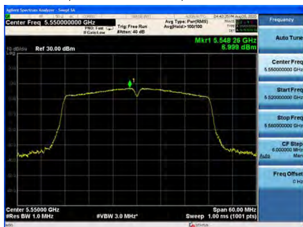
U-NII-2C, 802.11ac VHT40, Channel No.: 134
