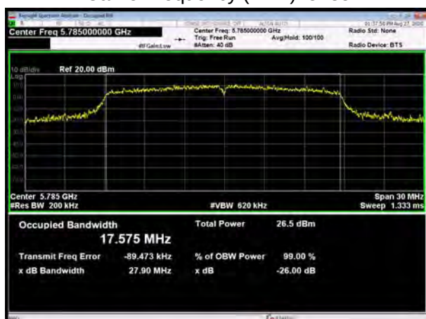
U-NII-3, 802.11n HT20 Carrier frequency (MHz): 5825
