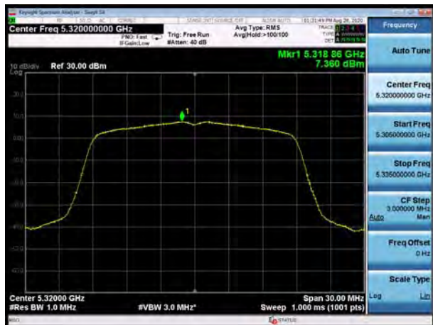
U-NII-2A, 802.11ac VHT20, Channel No.: 64
