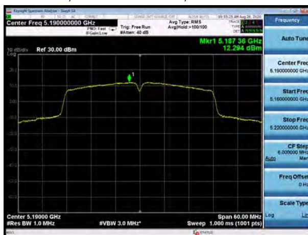
U-NII-1, 802.11ac VHT40, Channel No.: 38
