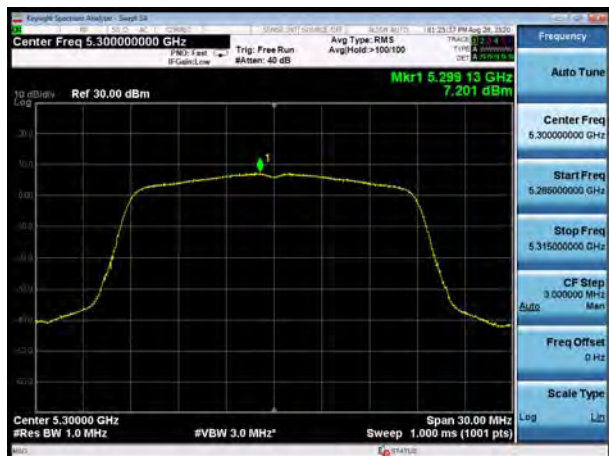
U-NII-2A, 802.11ac VHT20, Channel No.: 64
