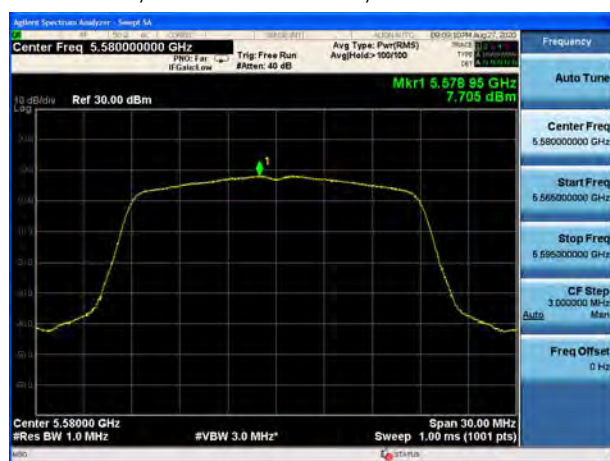
U-NII-2C, 802.11ac VHT20, Channel No.: 116
