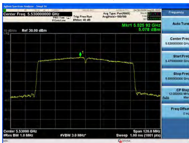
U-NII-2C, 802.11ac VHT80, Channel No.: 106
