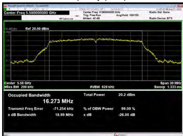
U-NII-2C, 802.11a Carrier frequency (MHz): 5700
