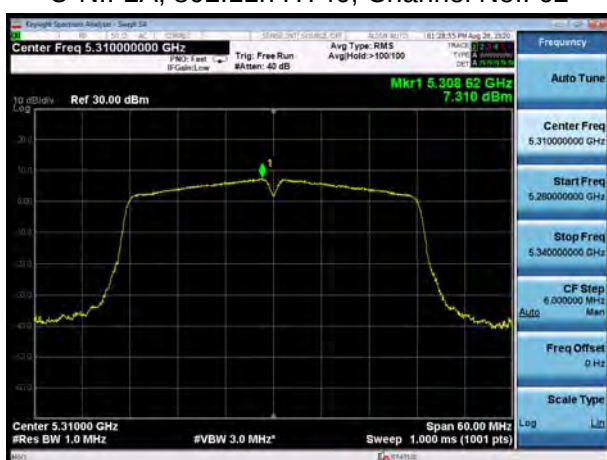
U-NII-2A, 802.11ac VHT40, Channel No.: 54
