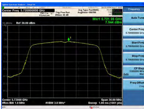
U-NII-2C, 802.11ac VHT80, Channel No.: 106
