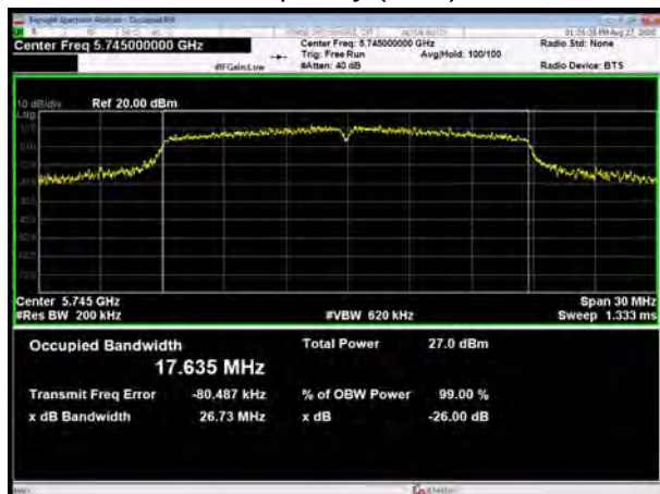
U-NII-3, 802.11n HT20 Carrier frequency (MHz): 5785
