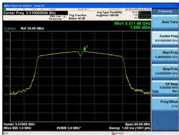
U-NII-2C, 802.11ac VHT40, Channel No.: 102
