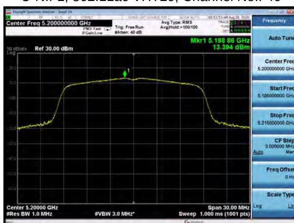
U-NII-1, 802.11ac VHT20, Channel No.: 48
