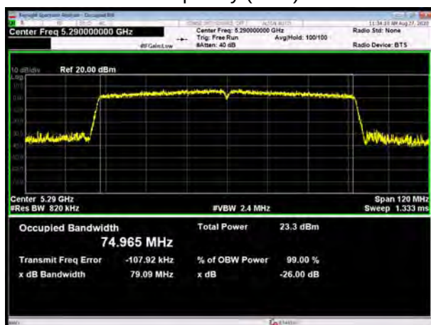
U-NII-2A, 802.11ax HE40 Carrier frequency (MHz): 5270
