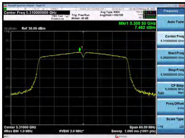
U-NII-2A, 802.11ac VHT80, Channel No.: 58
