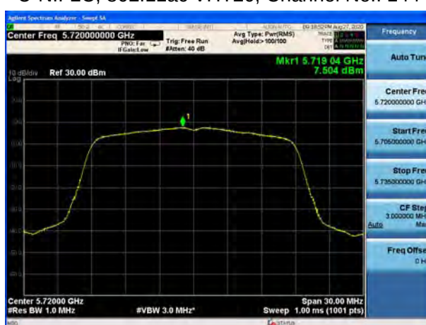
U-NII-2C, 802.11ac VHT80, Channel No.: 106
