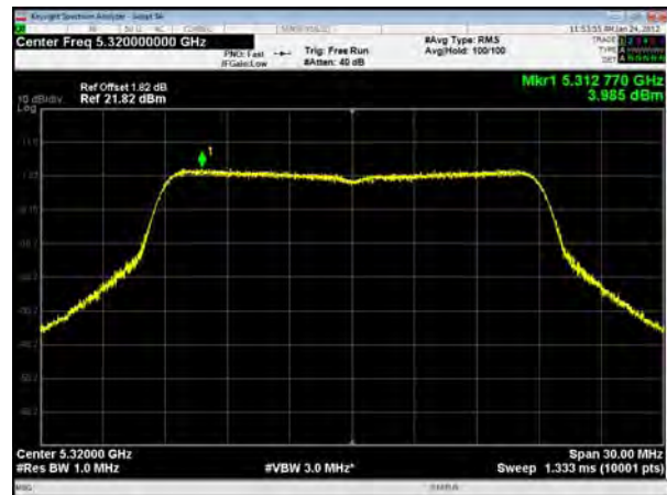
U-NII-2A, 802.11ac VHT20, Channel No.: 52
