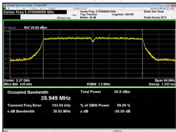
U-NII-2A, 802.11n HT40 Carrier frequency (MHz): 5310
