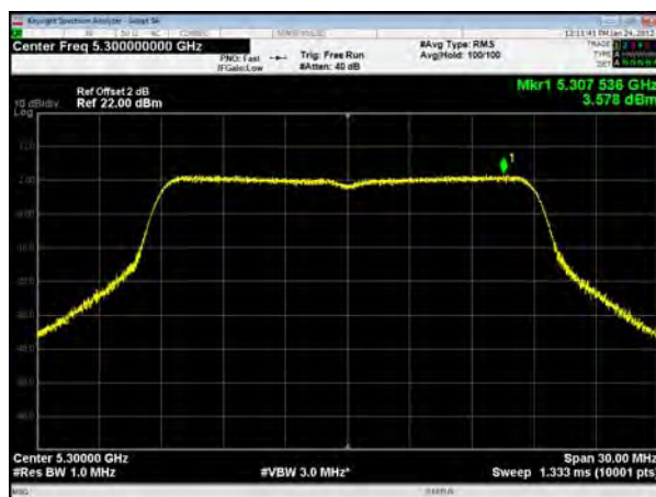
U-NII-2A, 802.11ac VHT20, Channel No.: 60
