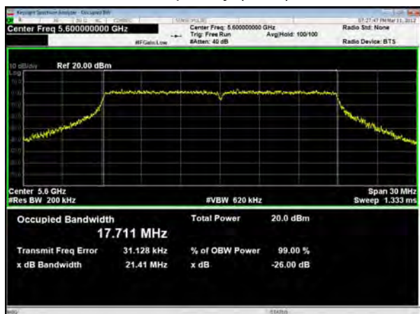
U-NII-2C, 802.11n HT20 Carrier frequency (MHz): 5700
