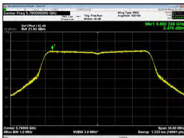
U-NII-2C, 802.11ac VHT20, Channel No.: 144
