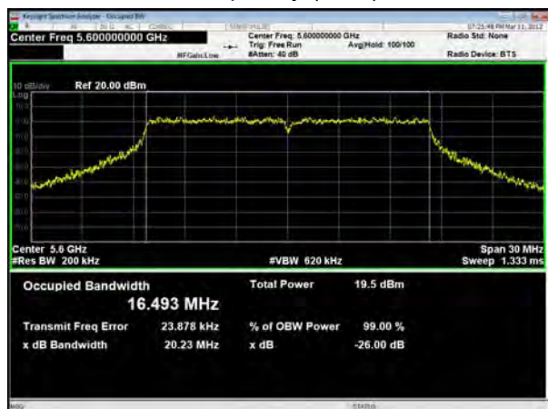
U-NII-2C, 802.11a Carrier frequency (MHz): 5700
