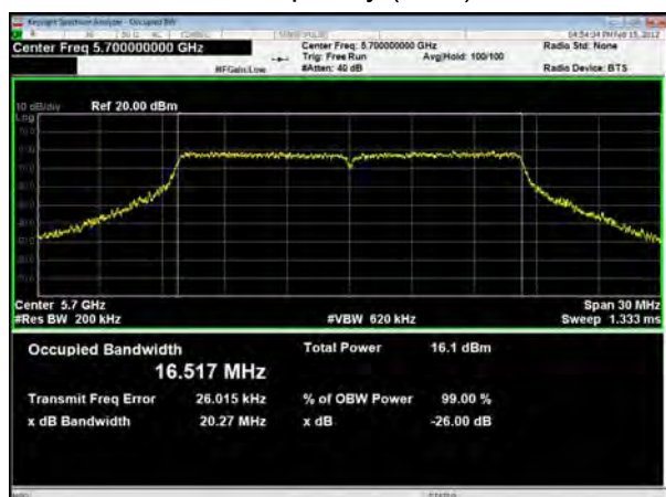
U-NII-2C, 802.11a Carrier frequency (MHz): 5700
