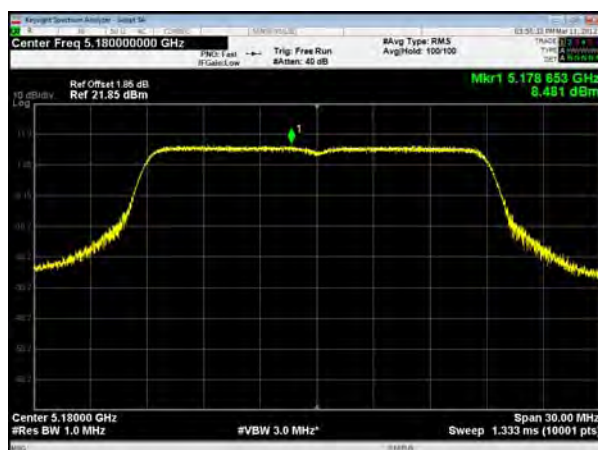
U-NII-1, 802.11ac VHT20, Channel No.: 40
