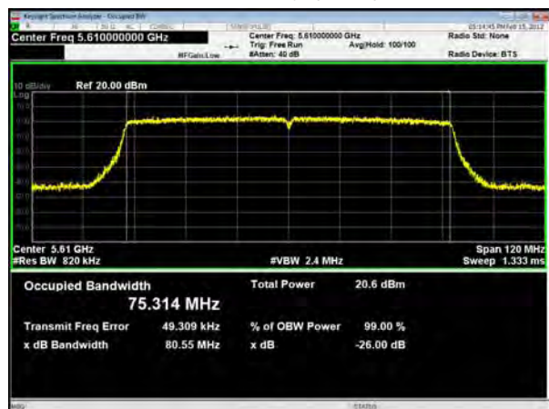
U-NII-2C, 802.11ac VHT80 Carrier frequency (MHz): 5690
