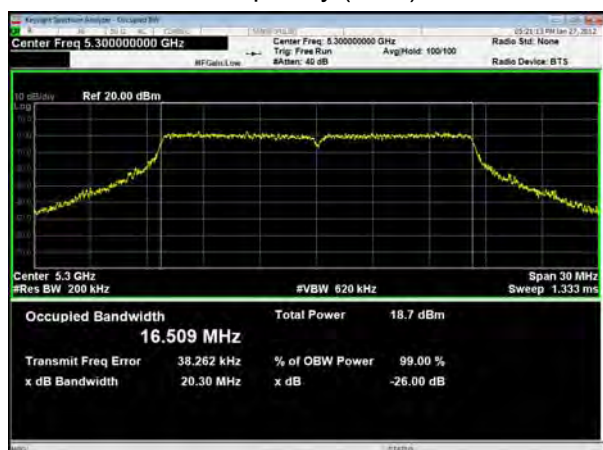
U-NII-2A, 802.11a Carrier frequency (MHz): 5300
