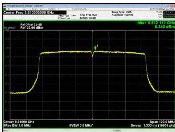
U-NII-2C, 802.11ac VHT80, Channel No.: 138
