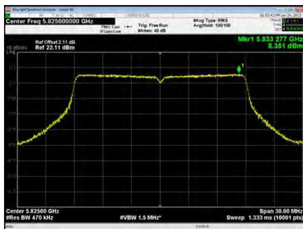
U-NII-3, 802.11ac VHT20, Channel No.: 165
