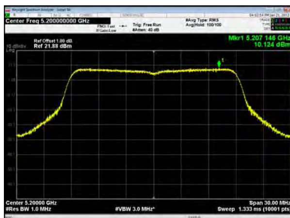
U-NII-1, 802.11ac VHT20, Channel No.: 48
