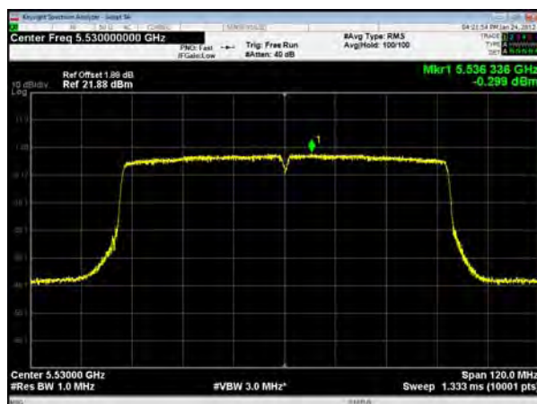
U-NII-2C, 802.11ac VHT80, Channel No.: 106
