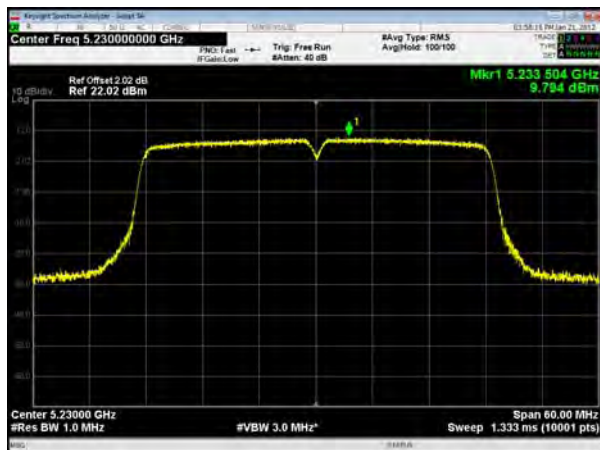
U-NII-1, 802.11ac VHT40, Channel No.: 38
