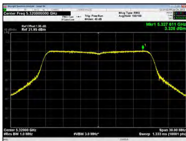
U-NII-2A, 802.11ac VHT80, Channel No.: 58
