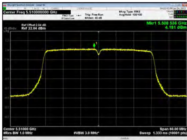
U-NII-2C, 802.11ac VHT40, Channel No.: 102
