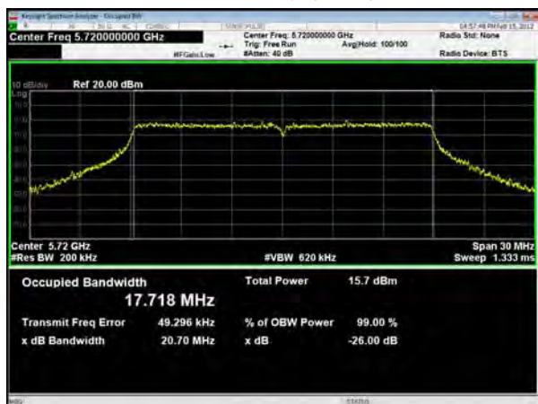
U-NII-2C, 802.11ac VHT20 Carrier frequency (MHz): 5500
