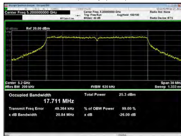
U-NII-1, 802.11ac VHT20 Carrier frequency (MHz): 5240
