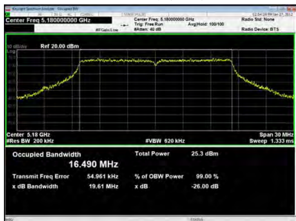
U-NII-1, 802.11a Carrier frequency (MHz): 5200
