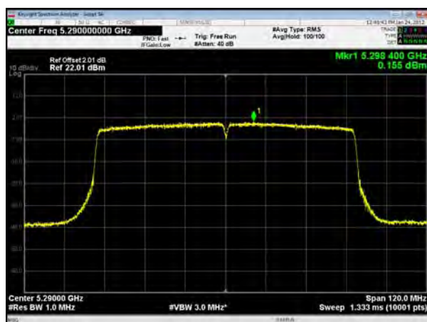
U-NII-2A, 802.11ac VHT160, Channel No.: 50
