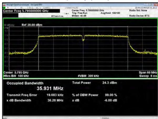
U-NII-3, 802.11ac VHT40 Carrier frequency (MHz): 5755
