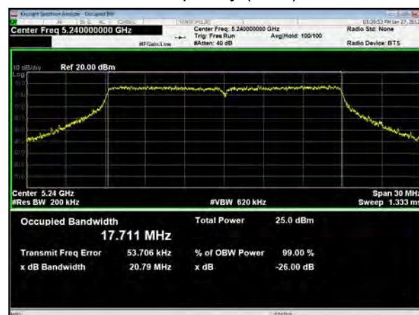
U-NII-1, 802.11ac VHT20 Carrier frequency (MHz): 5240
