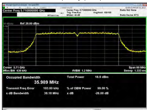
U-NII-2C, 802.11ac VHT40 Carrier frequency (MHz): 5710
