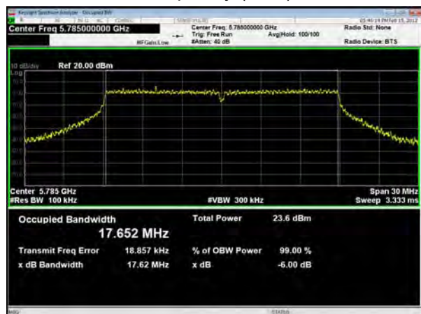
U-NII-3, 802.11ac VHT20 Carrier frequency (MHz): 5825
