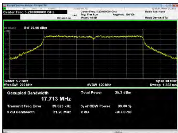
U-NII-1, 802.11n HT20 Carrier frequency (MHz): 5240
