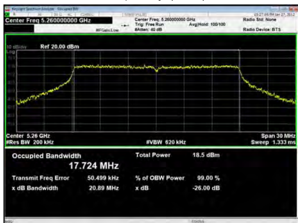
U-NII-2A, 802.11n HT20 Carrier frequency (MHz): 5300
