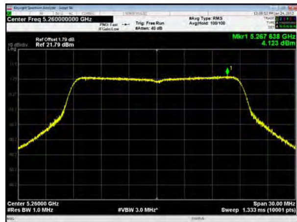
U-NII-2A, 802.11ac VHT20, Channel No.: 60
