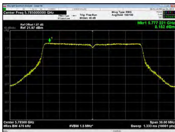
U-NII-3, 802.11ac VHT20, Channel No.: 165
