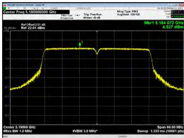
U-NII-1, 802.11ac VHT40, Channel No.: 38
