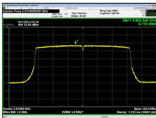
U-NII-2C, 802.11ac VHT80, Channel No.: 138
