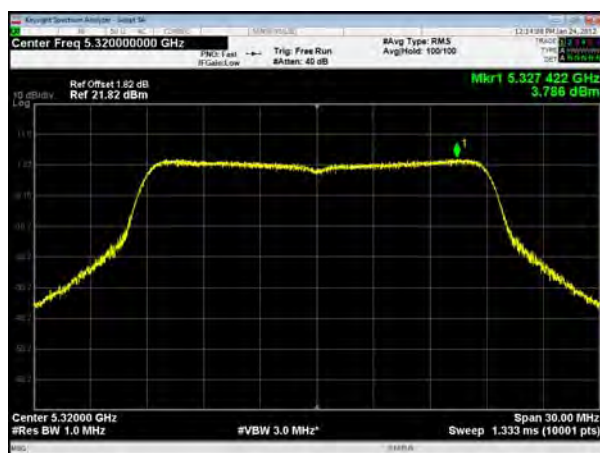
U-NII-2A, 802.11ac VHT80, Channel No.: 58
