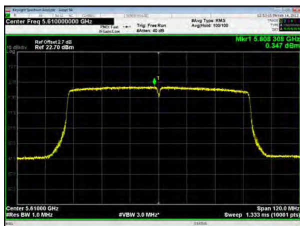
U-NII-2C, 802.11ac VHT80, Channel No.: 138
