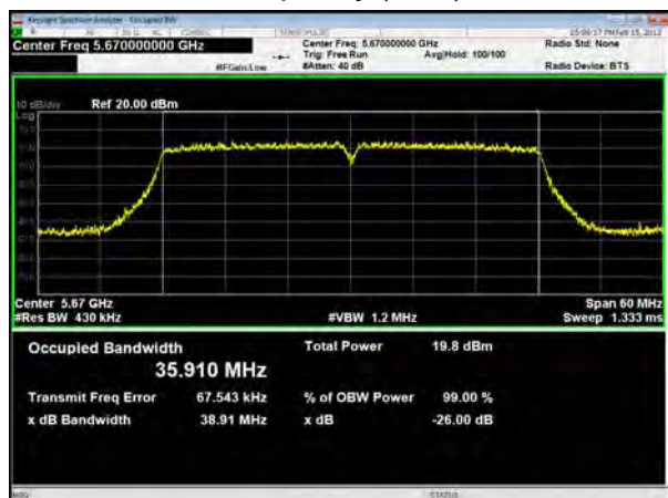
U-NII-2C, 802.11ac VHT40 Carrier frequency (MHz): 5710
