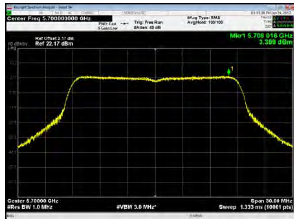
U-NII-2C, 802.11ac VHT20, Channel No.: 144
