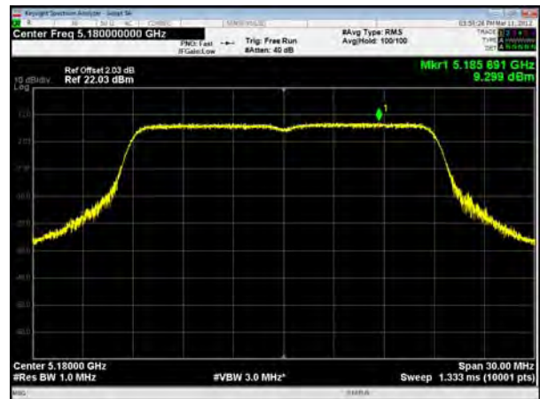
U-NII-1, 802.11ac VHT20, Channel No.: 40
