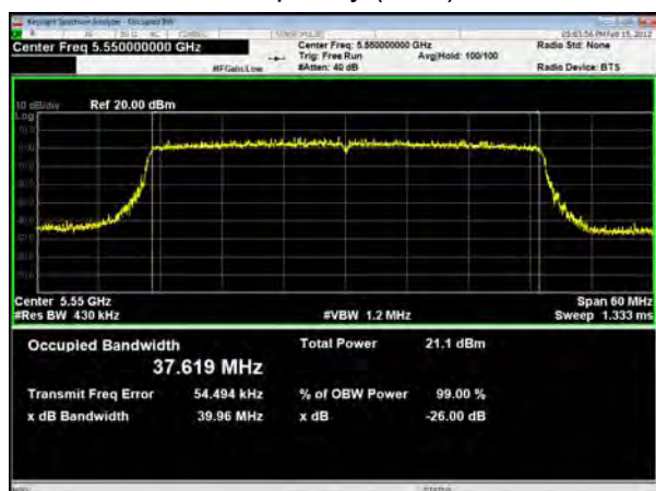
U-NII-2C, 802.11n HT40 Carrier frequency (MHz): 5550
