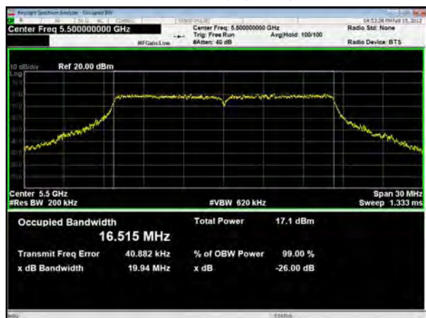
U-NII-2C, 802.11a Carrier frequency (MHz): 5600
