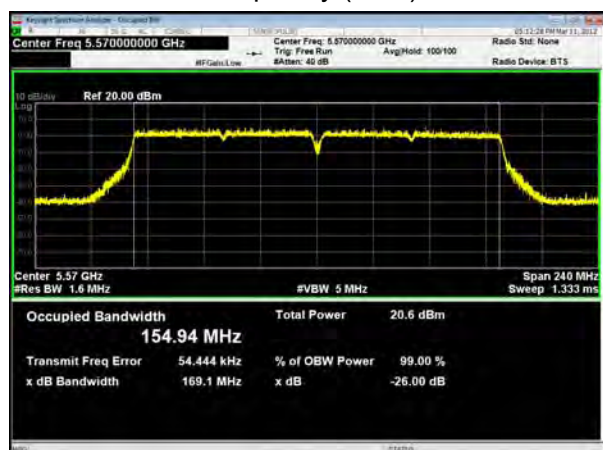
U-NII-2C, 802.11ac VHT160 Carrier frequency (MHz): 5570
