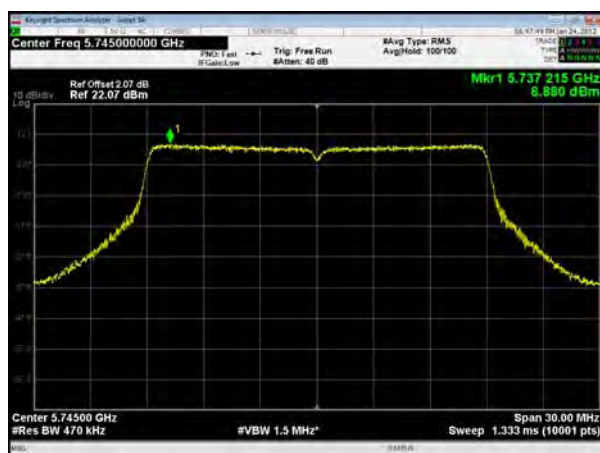
U-NII-3, 802.11ac VHT20, Channel No.: 157
