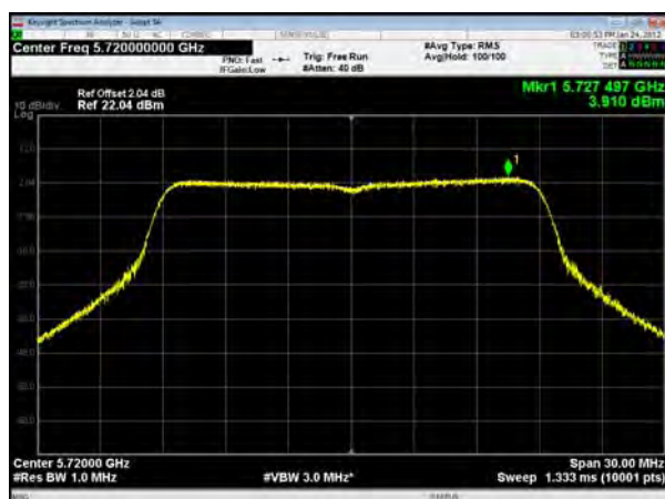
U-NII-2C, 802.11ac VHT20, Channel No.: 100
