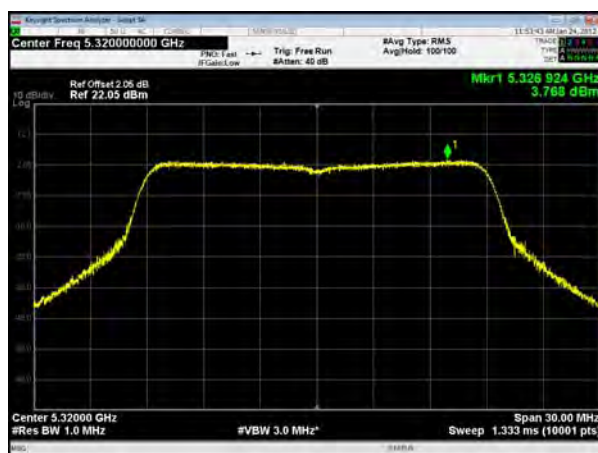
U-NII-2A, 802.11ac VHT20, Channel No.: 52
