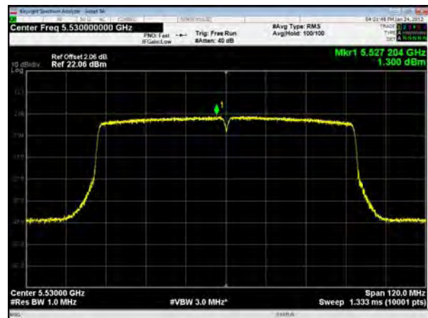
U-NII-2C, 802.11ac VHT80, Channel No.: 106
