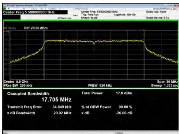
U-NII-2C, 802.11ac VHT20 Carrier frequency (MHz): 5600
