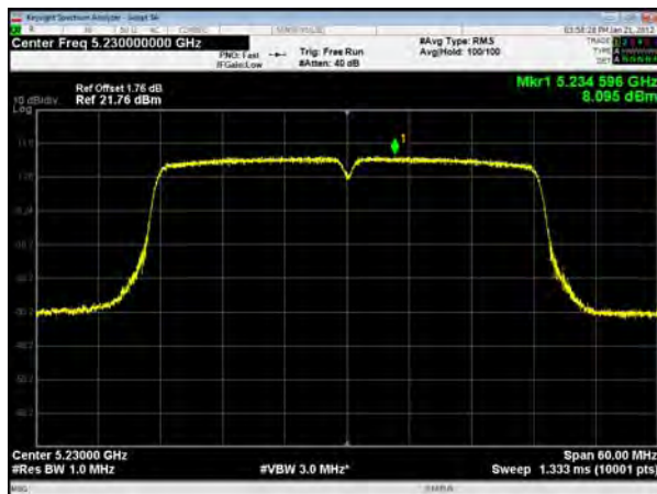
U-NII-1, 802.11ac VHT40, Channel No.: 38
