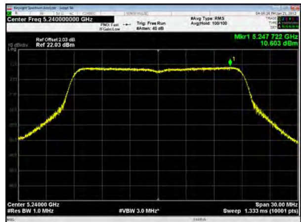
U-NII-1, 802.11ac VHT20, Channel No.: 48
