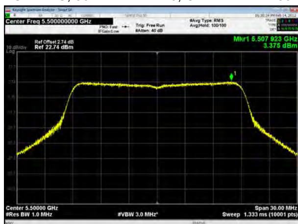
U-NII-2C, 802.11ac VHT20, Channel No.: 120
