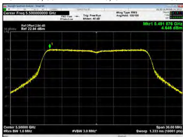
U-NII-2C, 802.11ac VHT20, Channel No.: 120
