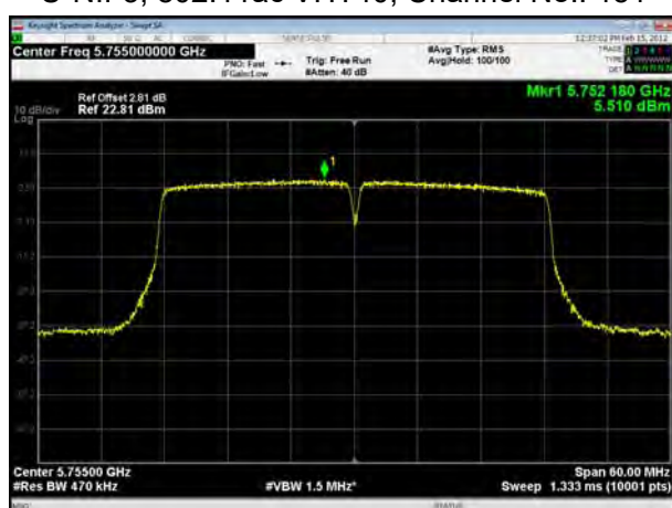
U-NII-3, 802.11ac VHT40, Channel No.: 159
