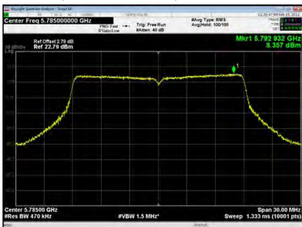
U-NII-3, 802.11ac VHT20, Channel No.: 157
