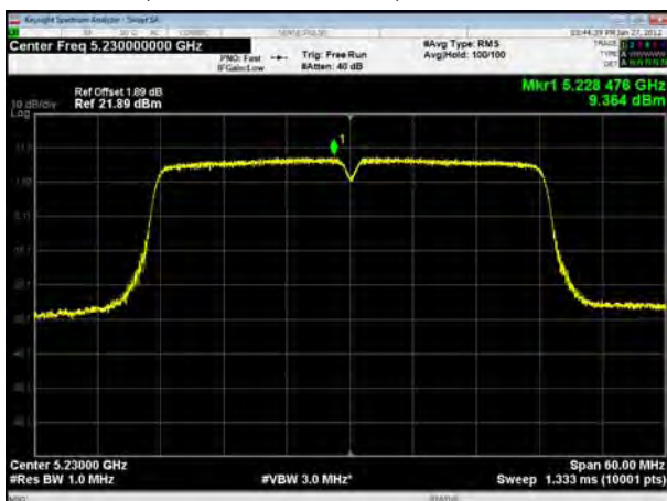
U-NII-1, 802.11ac VHT40, Channel No.: 46
