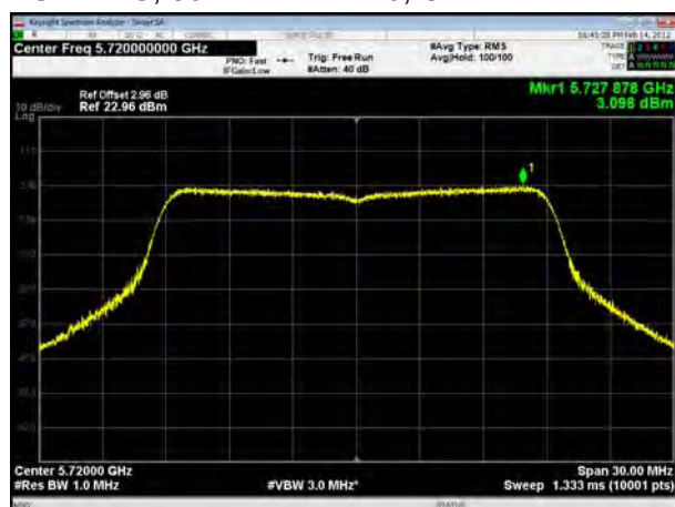
U-NII-2C, 802.11ac VHT40, Channel No.: 102
