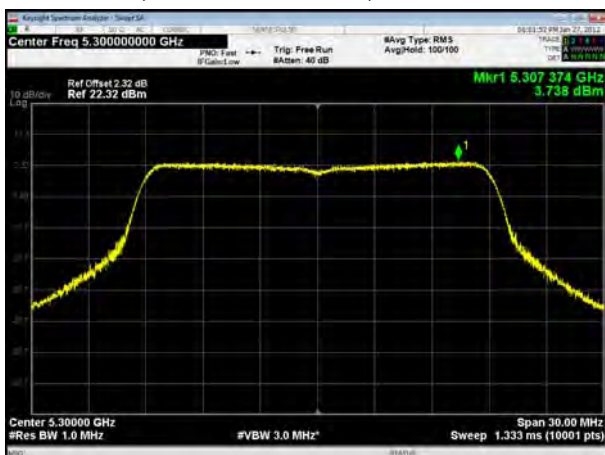
U-NII-2A, 802.11ac VHT20, Channel No.: 60
