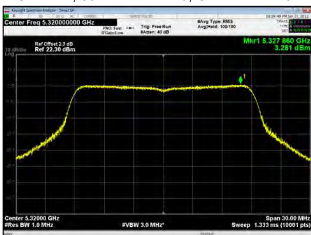
U-NII-2A, 802.11ac VHT40, Channel No.: 54
