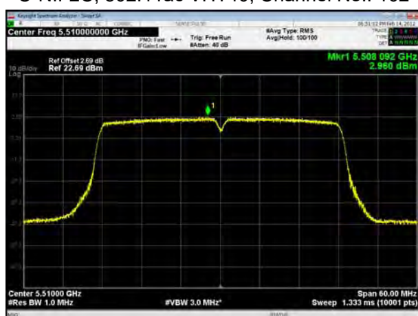
U-NII-2C, 802.11ac VHT40, Channel No.: 118
