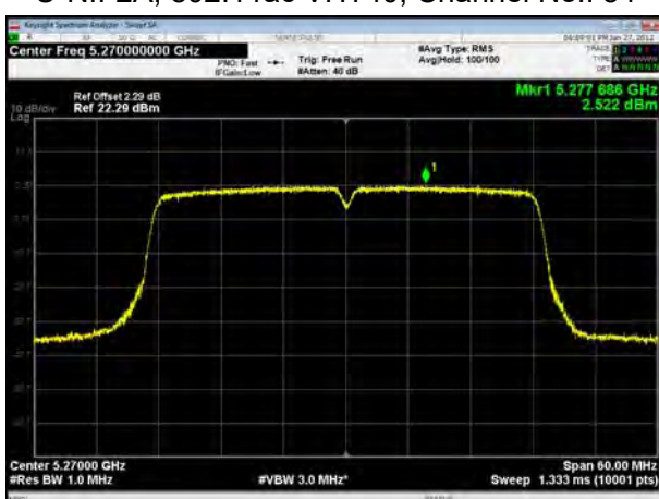
U-NII-2A, 802.11ac VHT40, Channel No.: 62
