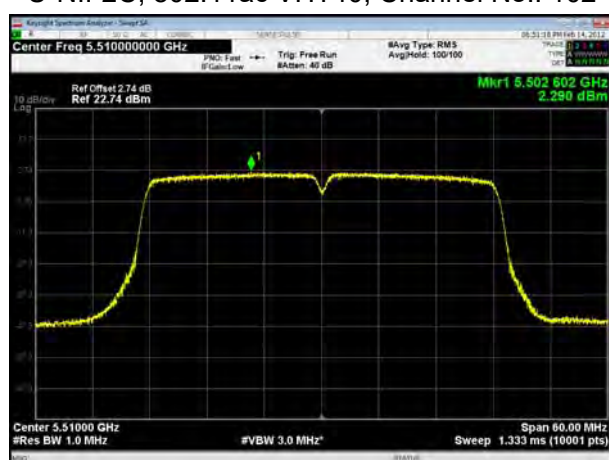
U-NII-2C, 802.11ac VHT40, Channel No.: 118
