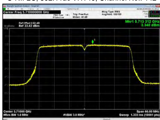
U-NII-2C, 802.11ac VHT80, Channel No.: 106
