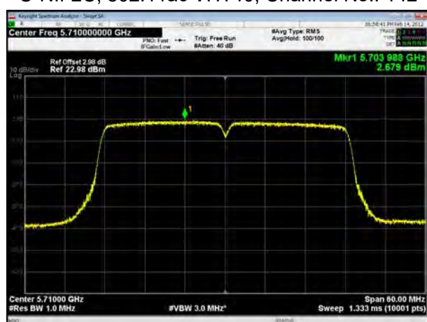
U-NII-2C, 802.11ac VHT80, Channel No.: 106
