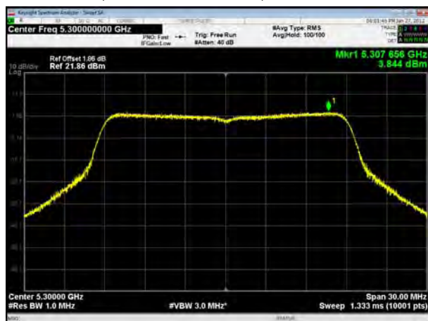
U-NII-2A, 802.11ac VHT20, Channel No.: 60
