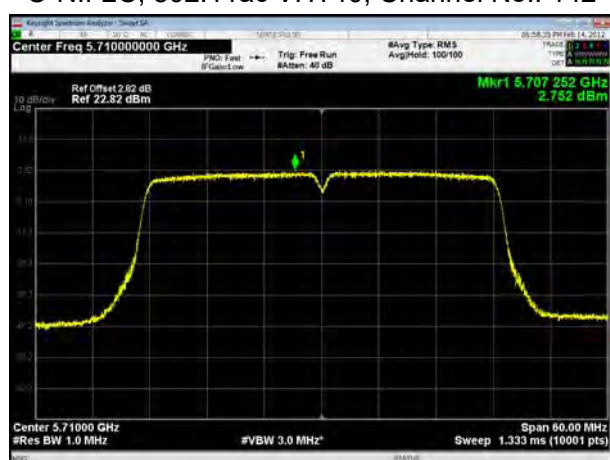
U-NII-2C, 802.11ac VHT80, Channel No.: 106
