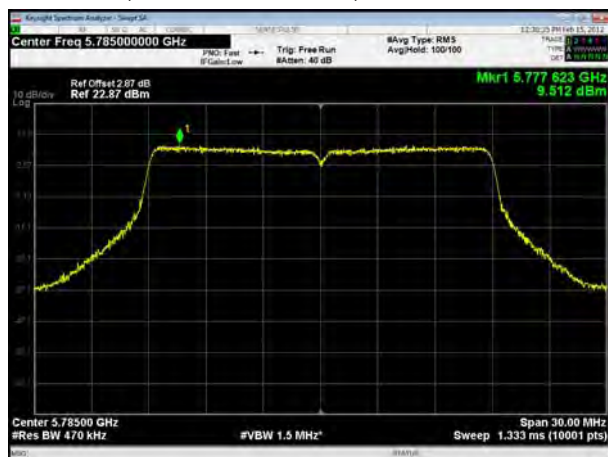
U-NII-3, 802.11ac VHT20, Channel No.: 157
