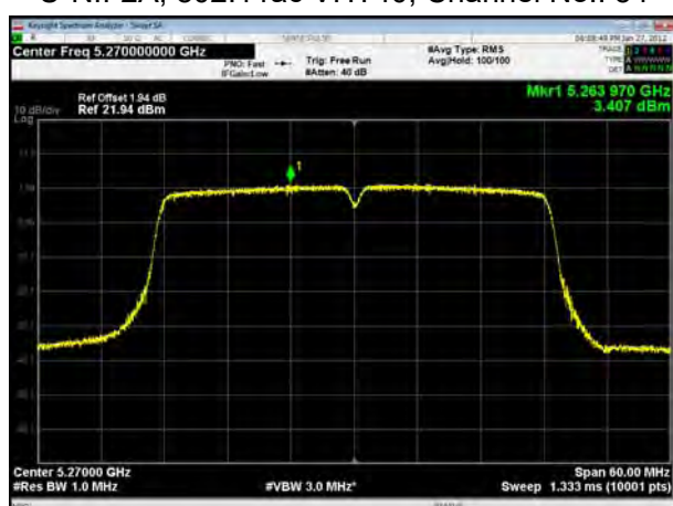
U-NII-2A, 802.11ac VHT40, Channel No.: 62
