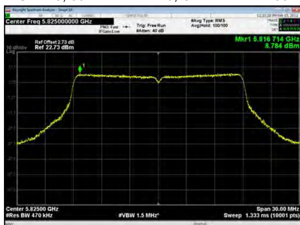
U-NII-3, 802.11ac VHT40, Channel No.: 151
