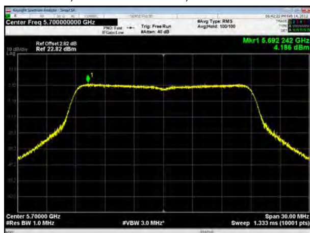
U-NII-2C, 802.11ac VHT20, Channel No.: 140
