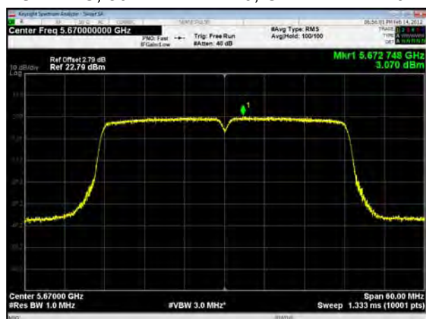
U-NII-2C, 802.11ac VHT40, Channel No.: 142
