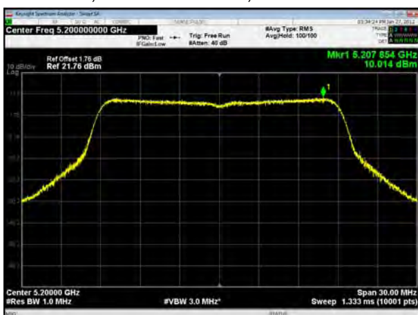
U-NII-1, 802.11ac VHT20, Channel No.: 40
