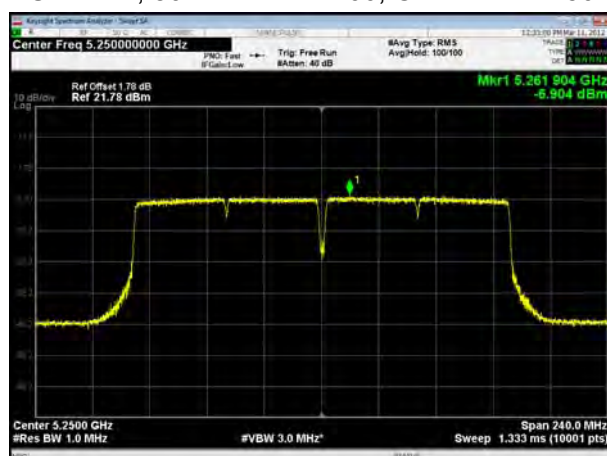
U-NII-2A, 802.11ac VHT160, Channel No.: 50
