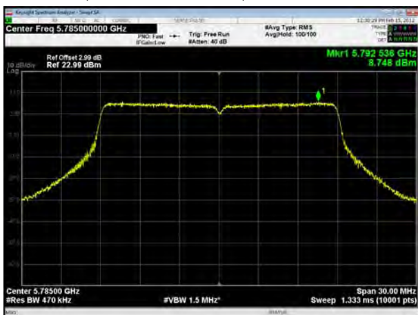
U-NII-3, 802.11ac VHT20, Channel No.: 157
