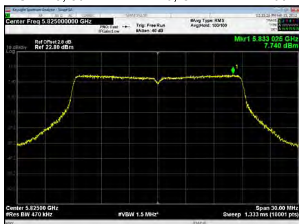
U-NII-3, 802.11ac VHT40, Channel No.: 151
