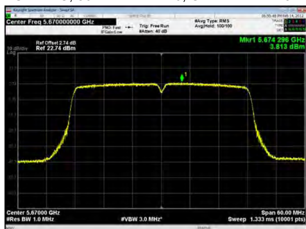
U-NII-2C, 802.11ac VHT40, Channel No.: 142
