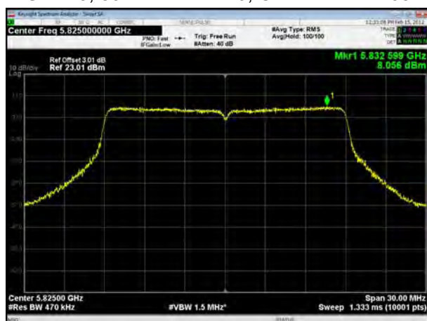
U-NII-3, 802.11ac VHT40, Channel No.: 151
