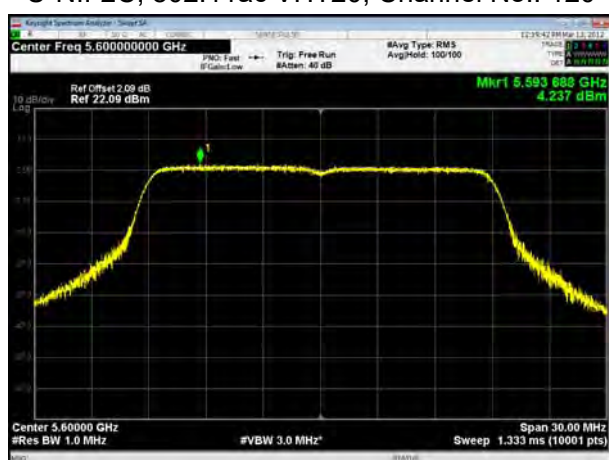
U-NII-2C, 802.11ac VHT20, Channel No.: 140
