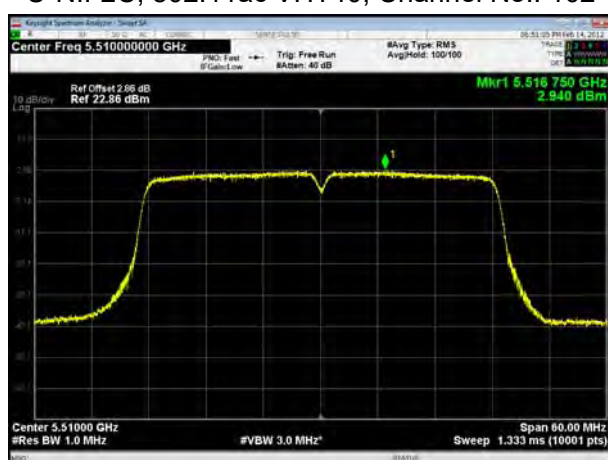
U-NII-2C, 802.11ac VHT40, Channel No.: 118
