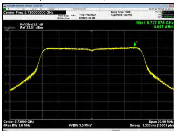
U-NII-2C, 802.11ac VHT40, Channel No.: 102
