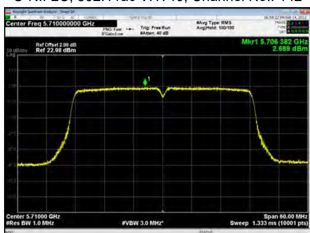
U-NII-2C, 802.11ac VHT80, Channel No.: 106
