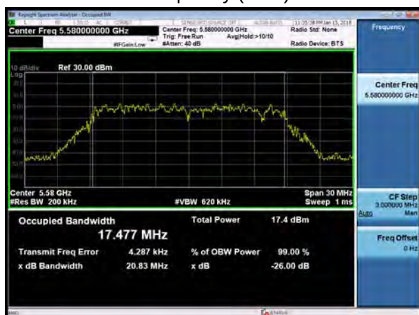
U-NII-2C, 802.11n HT20 Carrier frequency (MHz): 5700
