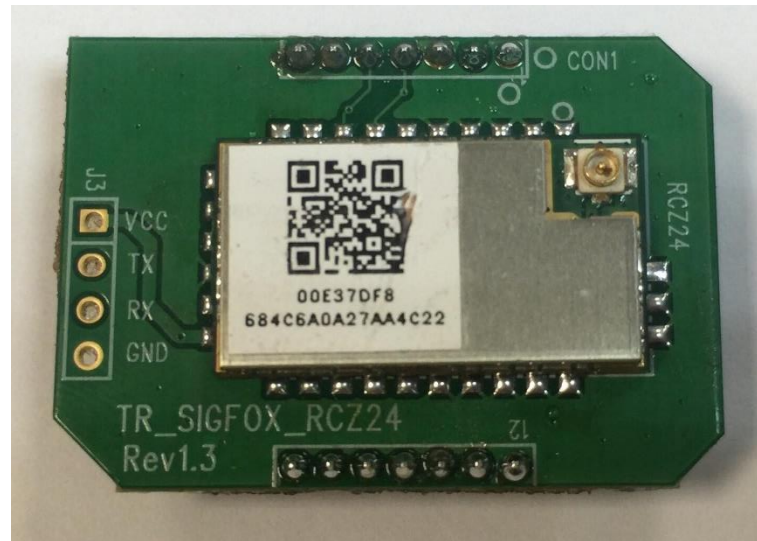
Fig.4 Module_Sigfox_RCZ2 on the carrier board
