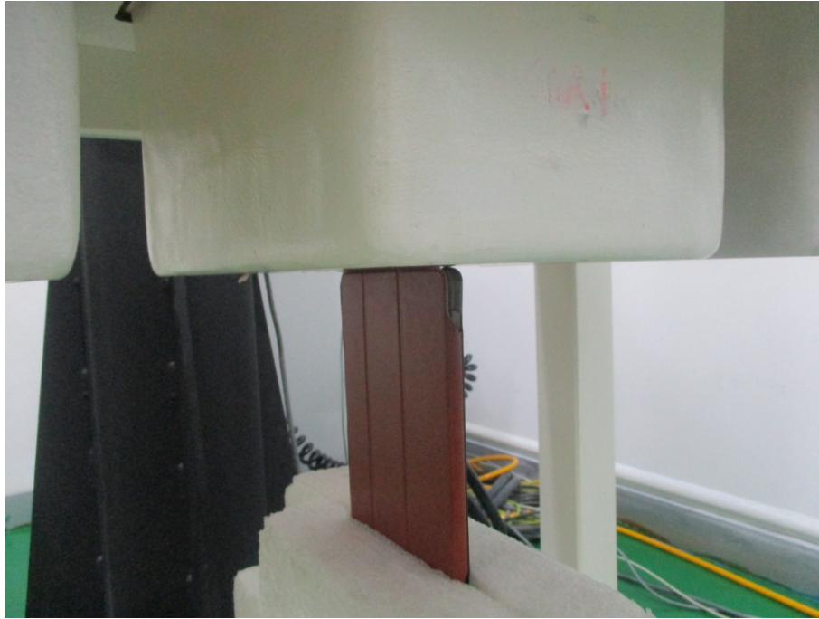
Body Bottom Setup Photo(0mm)
