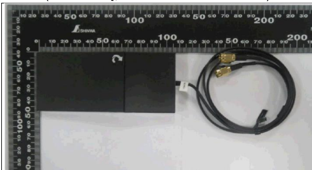
Antenna set 2 (Brand : INPAQ, Model : DAM-I6-H-DB-800-10-17)
