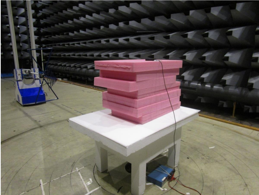
Photo 4.1.1 Test setup regarding measurement of radiated emission.
