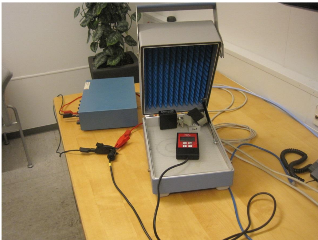
Photo 4.4.1 Test setup regarding measurement of 20 dB bandwidth.
