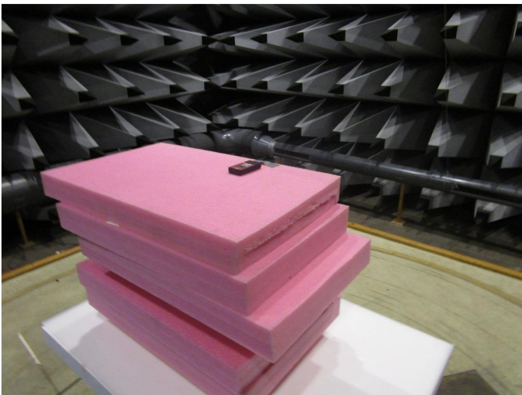
Photo 4.1.2 Test setup regarding measurement of radiated emission.
