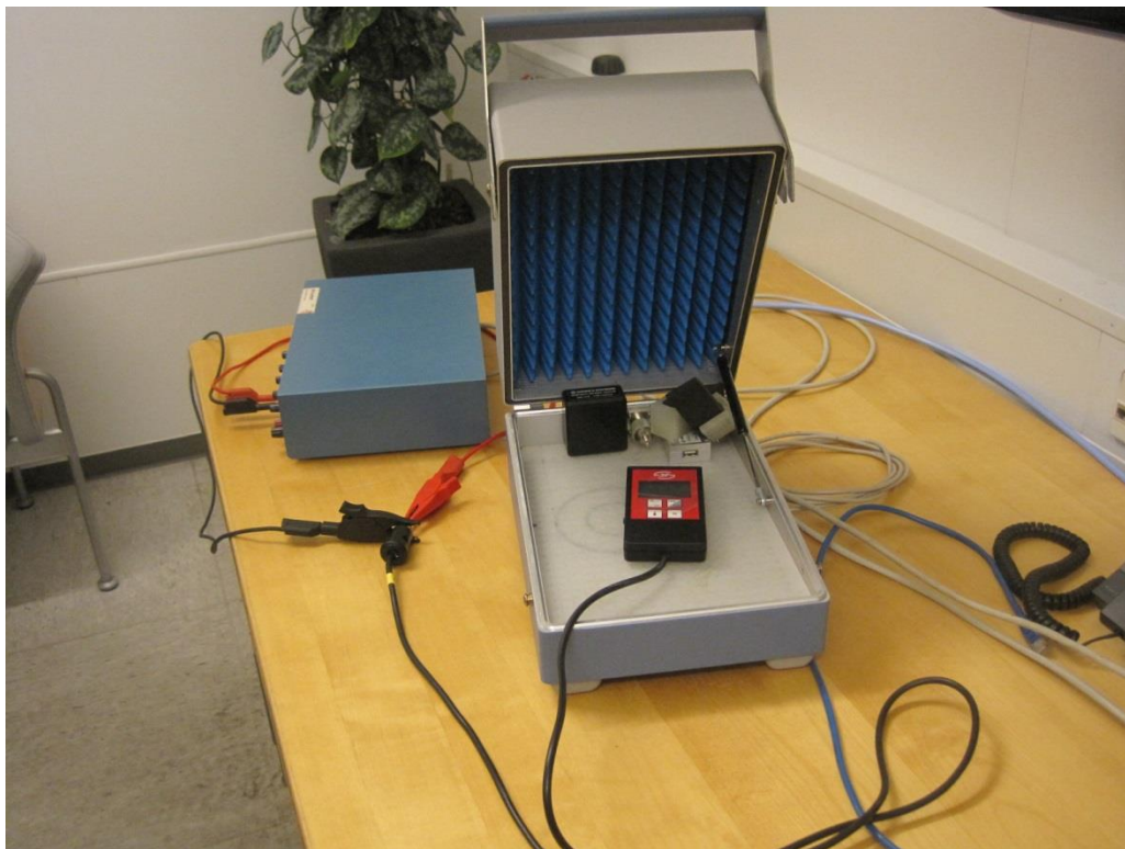
Photo 4.5.1 Test setup regarding measurement of occupied bandwidth, IC.
