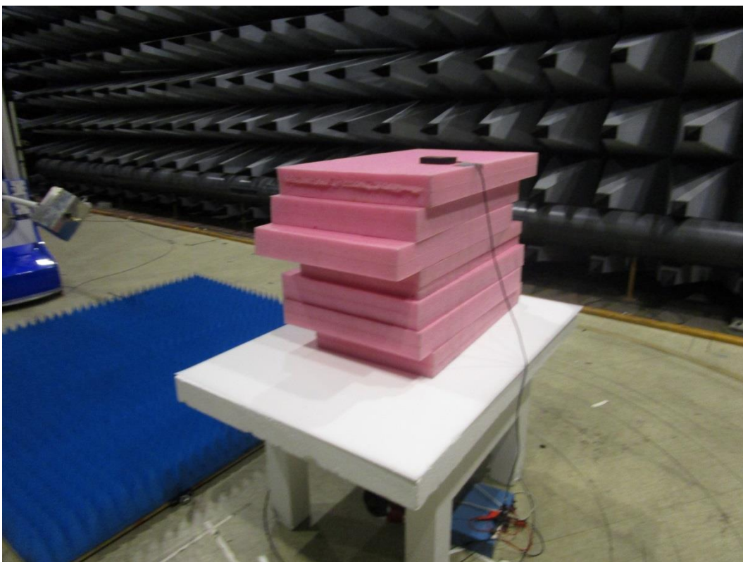
Photo 4.1.4 Test setup regarding measurement of radiated emission.
