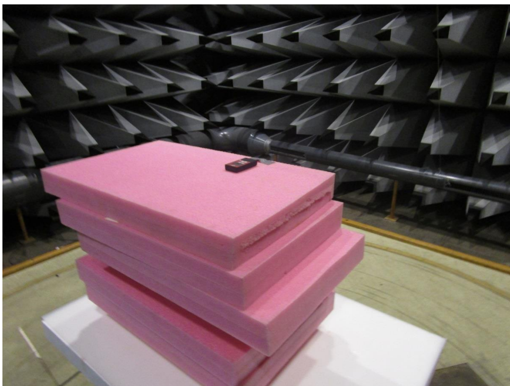
Photo4.3.2 Test setup regarding measurement of band edge compliance.
