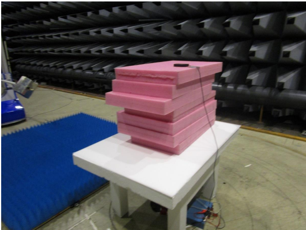
Photo 4.1.4 Test setup regarding measurement of radiated emission.
