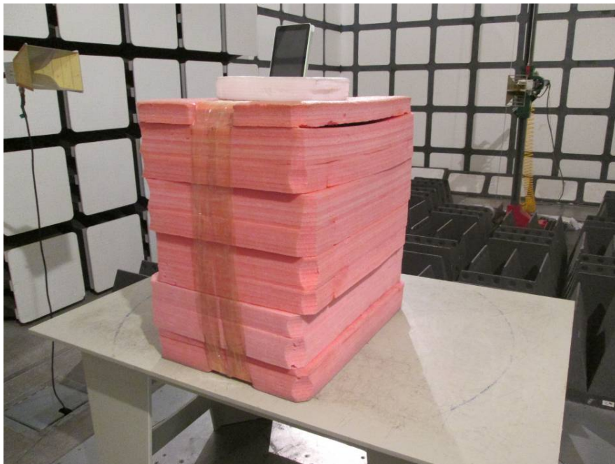
Radiated Emissions Test View (Above 1 GHz)
