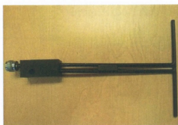
Figure 1 – MVG COMOSAR Validation Dipole
