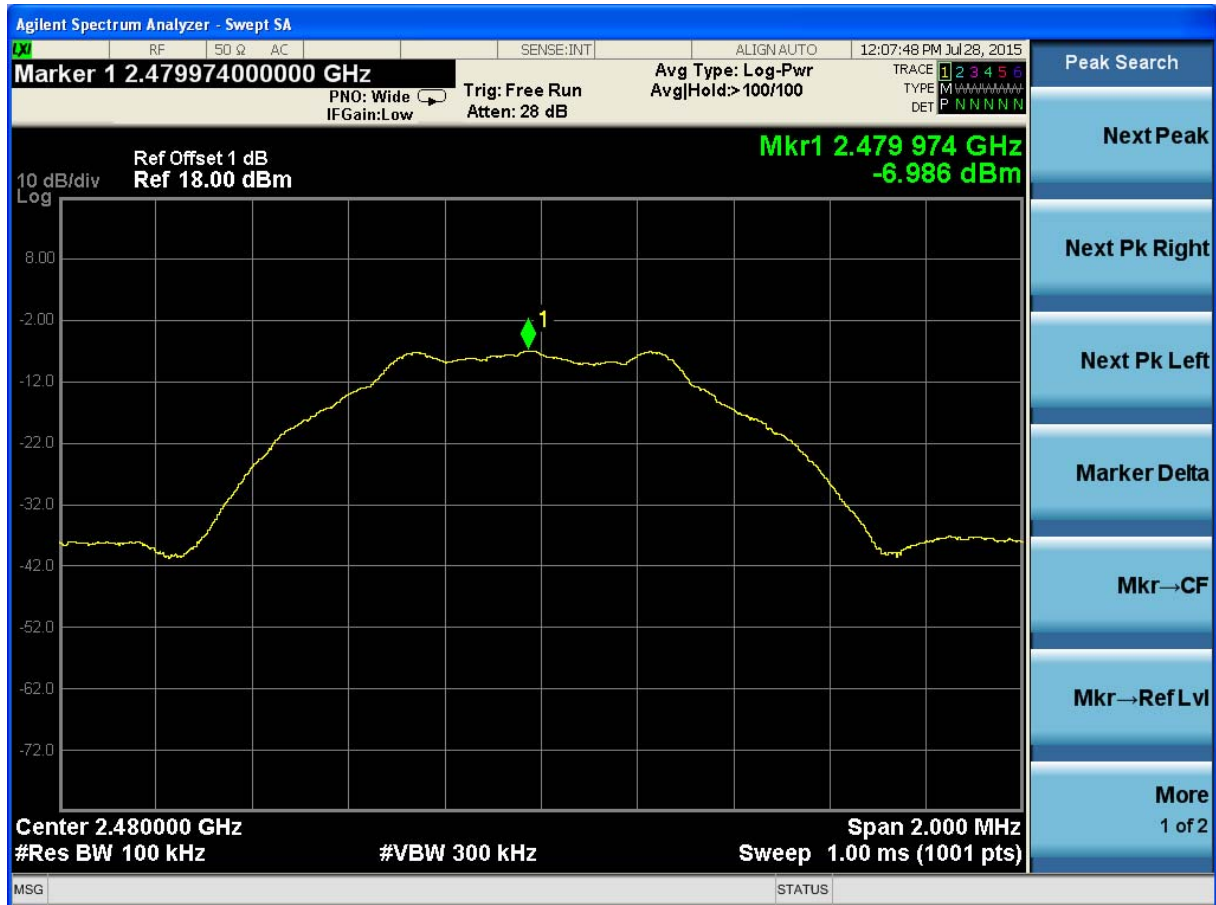
(Plot 4.4.1 C : Channel 39: 2480MHz @ GFSK)
