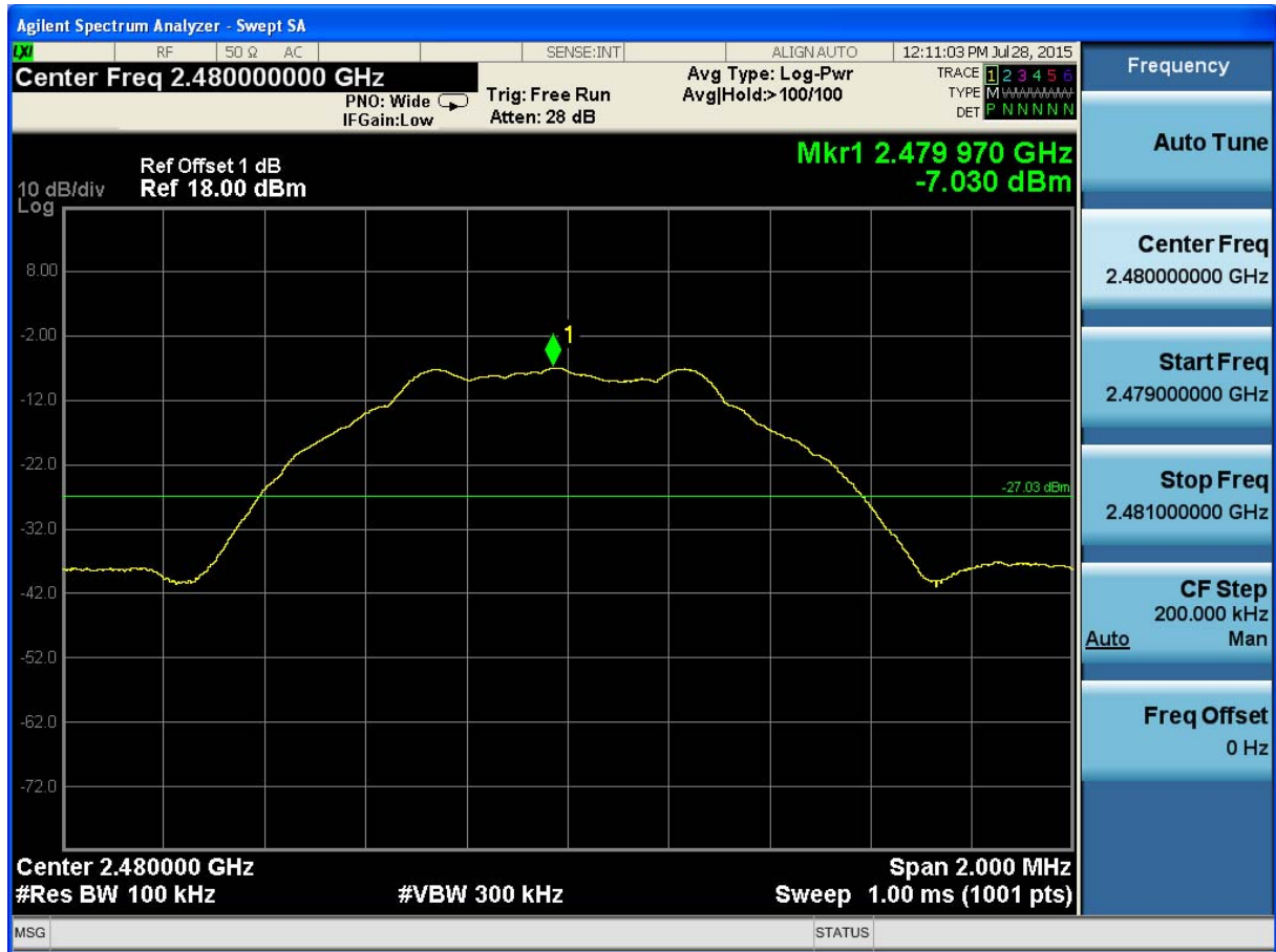
(Plot 4.7.1 C1: Channel 39: 2480MHz @ GFSK)
