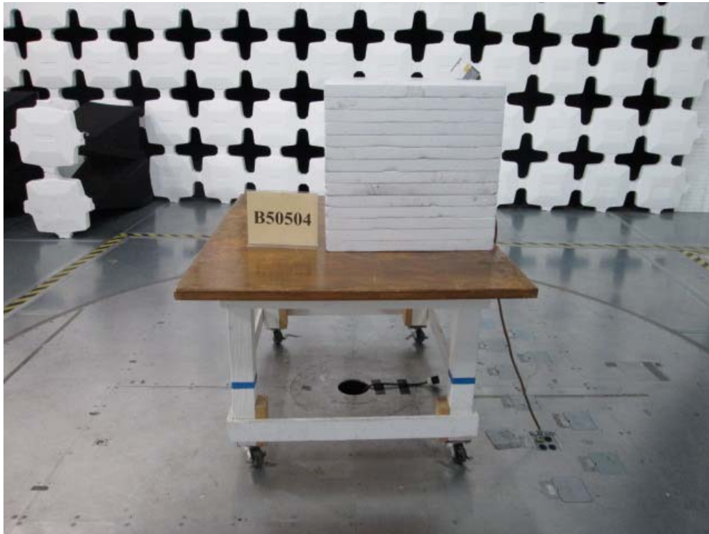
Figure A17: Radiated Emissions Test Setup - Right
