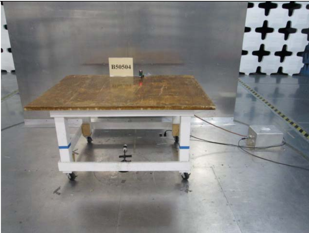
Figure B7: Conducted Emissions Test Setup - Front
