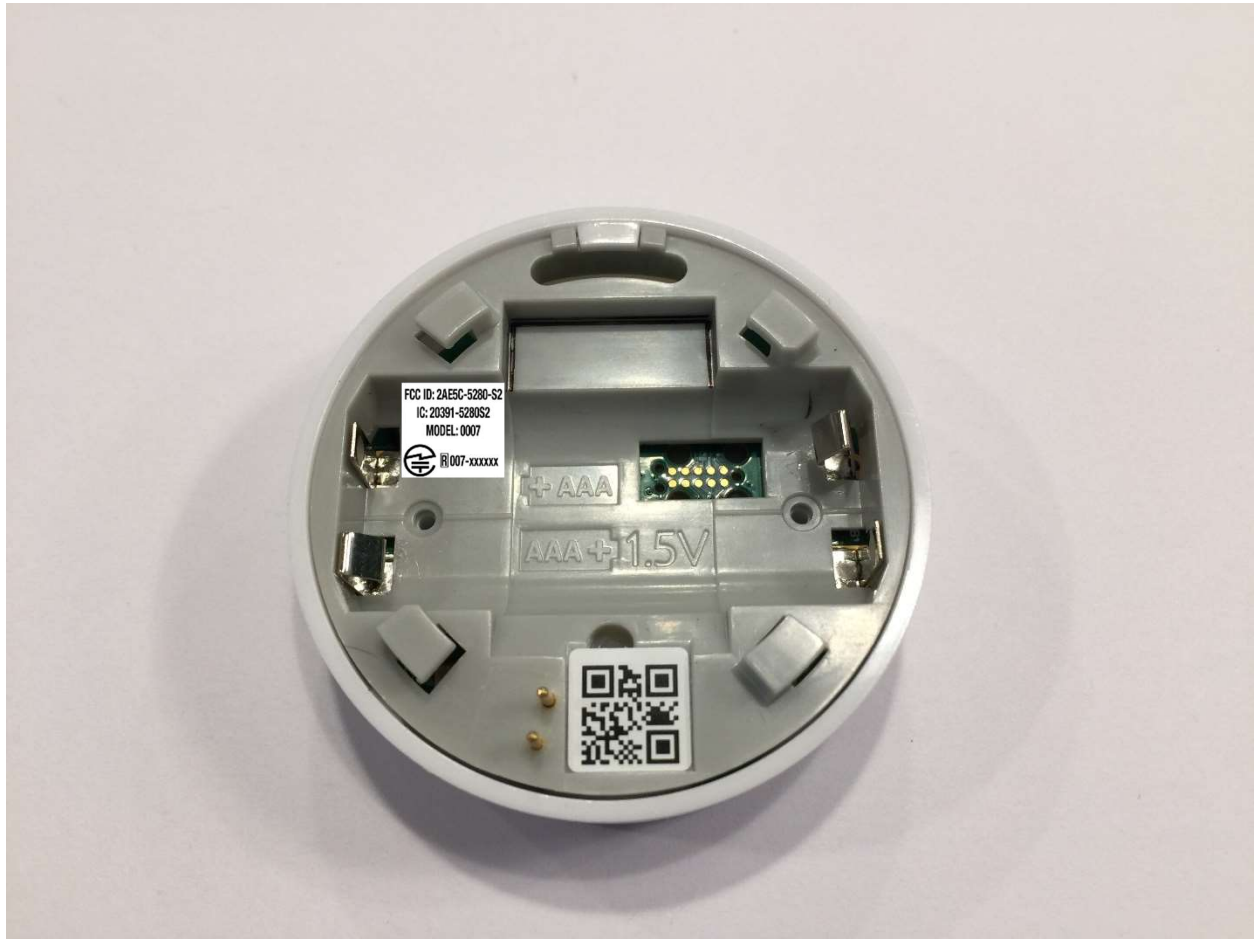
Figure 1- Granite Sensor, (Internal) Battery Cover View
