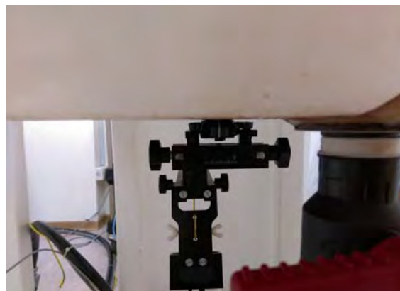
Fig.3 EUT Front side_1 to flat phantom
