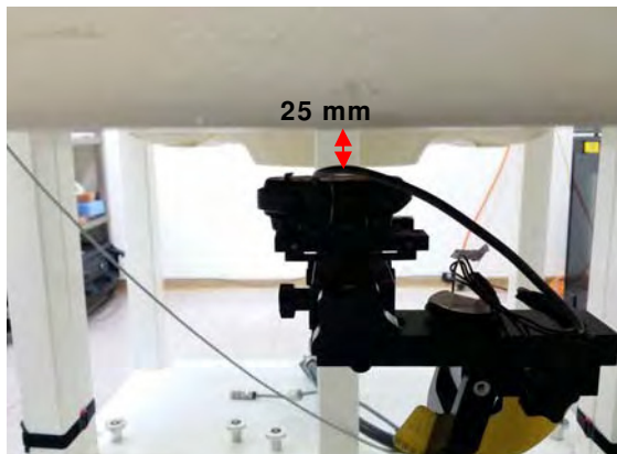
Fig.14 EUT Back side with headset to flat phantom
