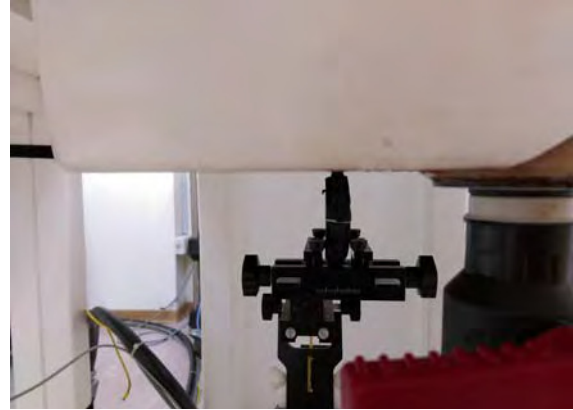
Fig.12 EUT Right side to flat phantom
