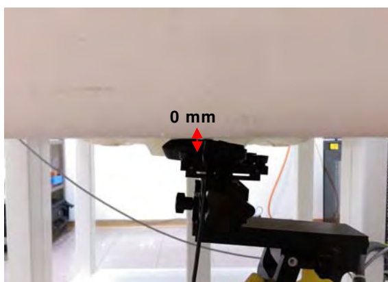
Fig.4 EUT Front side_1 with headset to flat phantom
