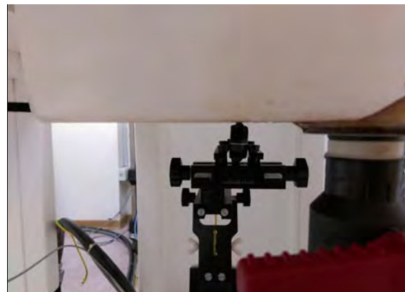
Fig.10 EUT Top side to flat phantom
