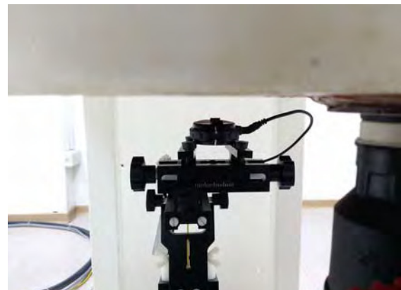
Fig.14 EUT Back side with headset to flat phantom
