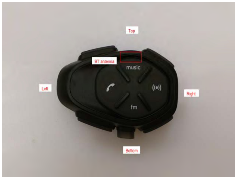
Fig.18 Antenna position of EUT (Front view)
