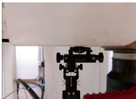
Fig.5 EUT Front side_2 to flat phantom
