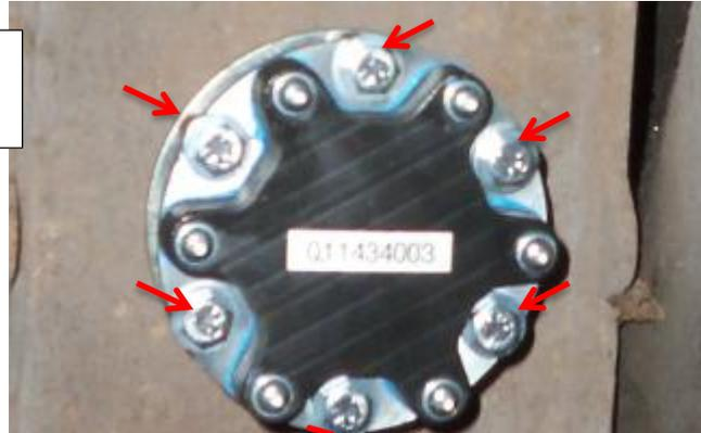
Figure 2.5: Sensor Bolts Installation
