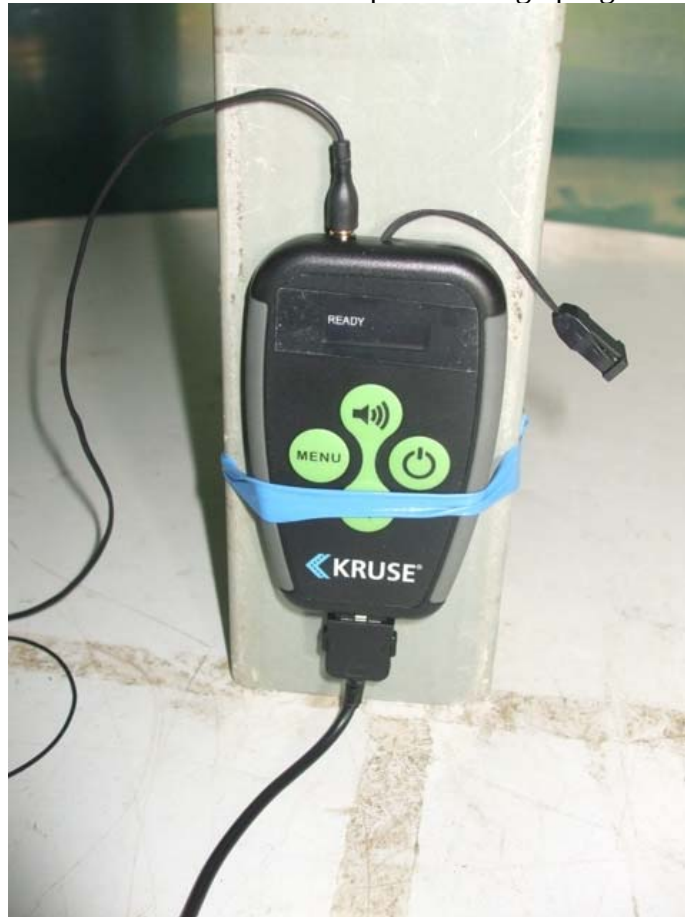
Radiated emissions setup – Standing up right
