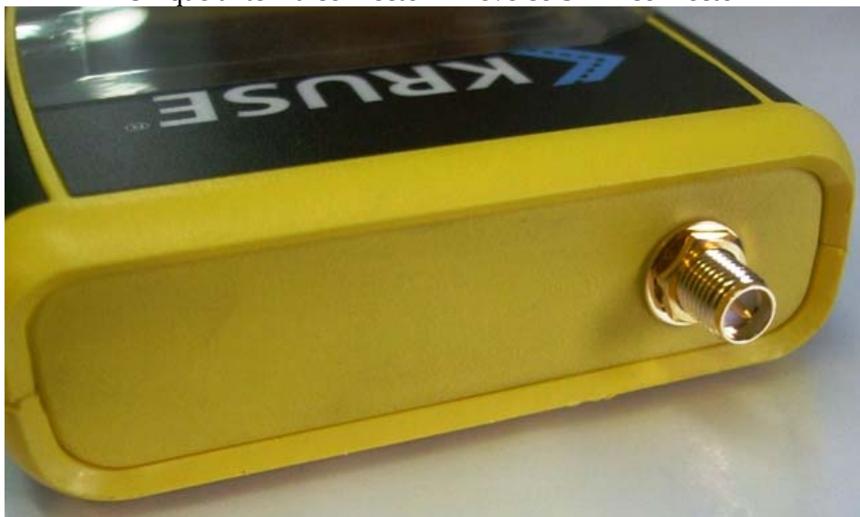
Unique antenna connector – Reverse SMA connector
