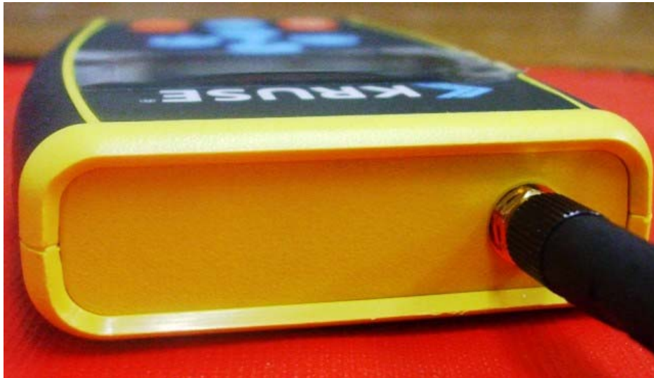
Unique antenna connector – Reverse SMA connector
