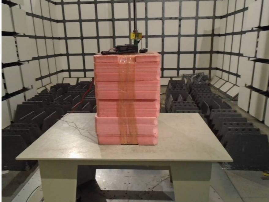
Transmitting Radiated Emissions Front View (Above 1 GHz)
