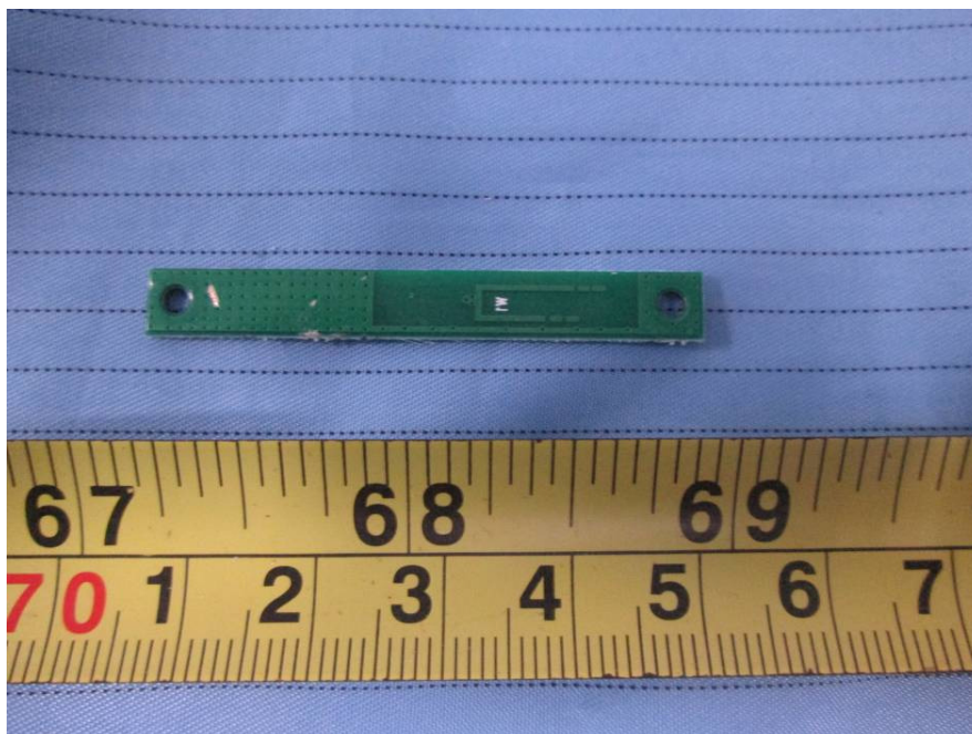
EUT – BT & GPS Antenna Bottom View
