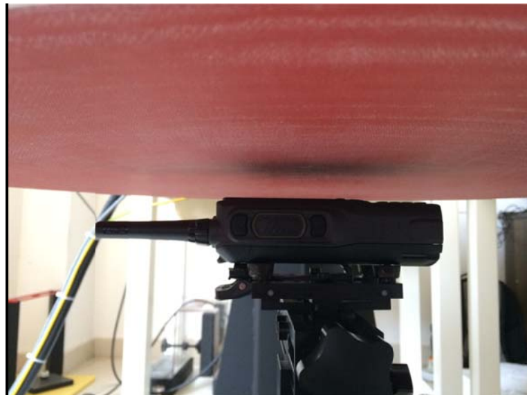
25mm Face-held, The EUT display towards phantom
