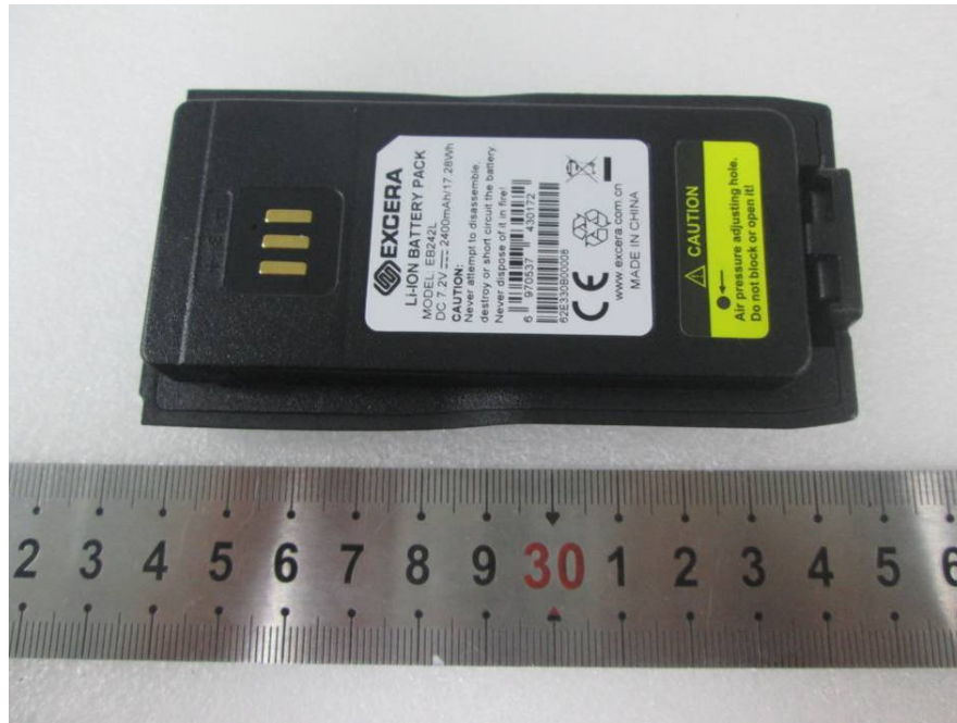
EUT (EP8000 U2) –Battery View
