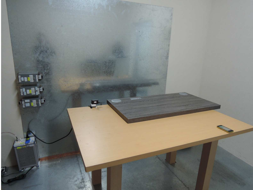
Photograph 6: Set-up for for Mains Conducted testing Front
