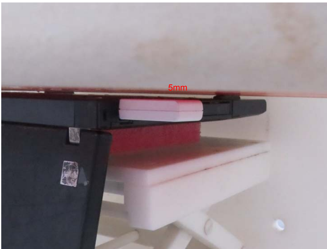
Picture 6: Front Side, the distance from EUT to the bottom of the Phantom is 5mm
