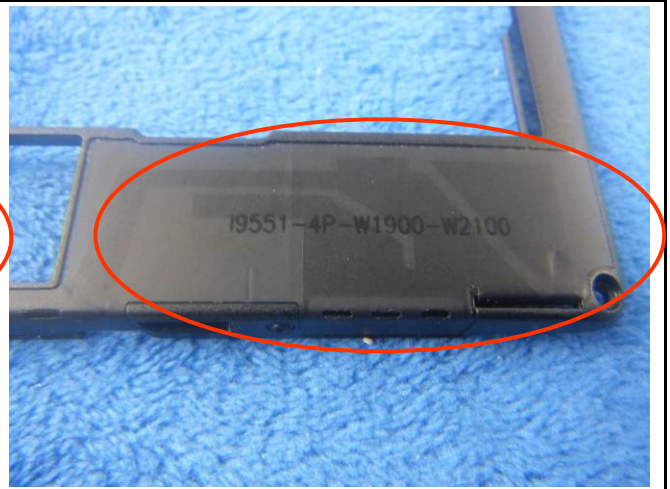
GSM/PCS/UMTS-FDD Antenna View
