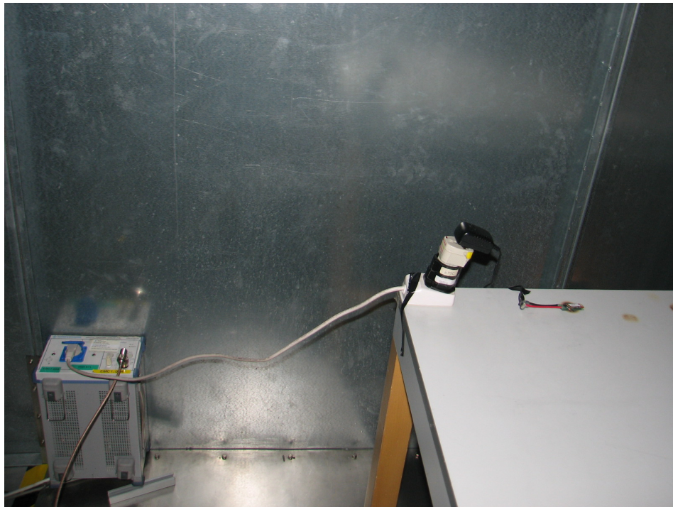
Setup for Disturbance voltage on AC mains
