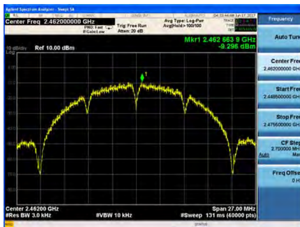
(802.11b) PSD plot on channel 11
