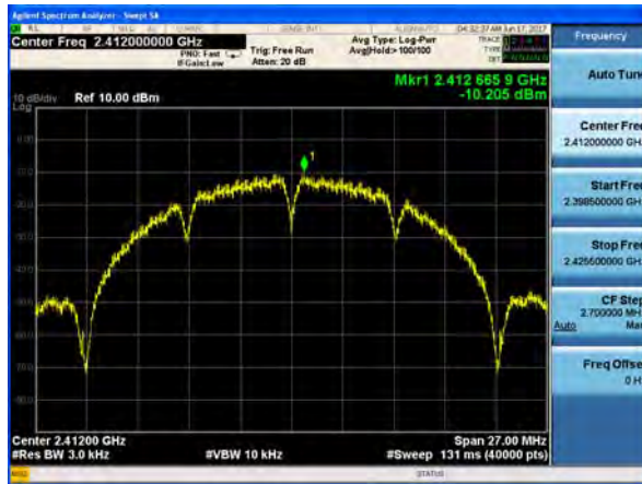
(802.11b) PSD plot on channel 6
