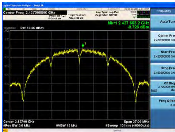
(802.11b) PSD plot on channel 6
