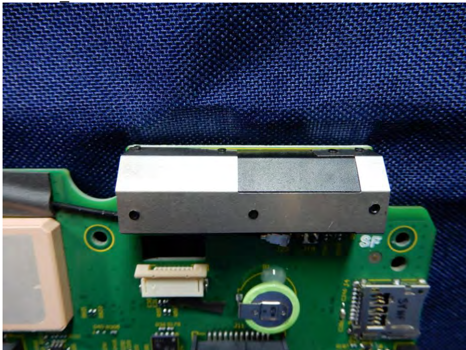
(36) EUT Photo WWAN Aux Ant
