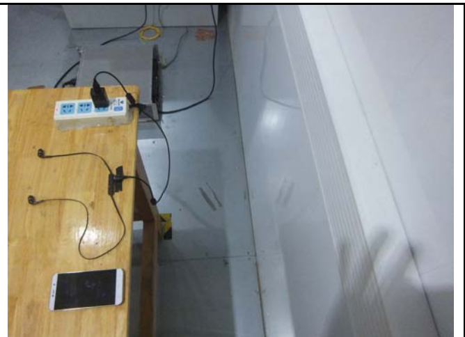
Conducted Emissions Test Setup Side View
