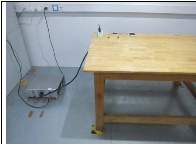
Conducted Emissions Test Setup Front View
