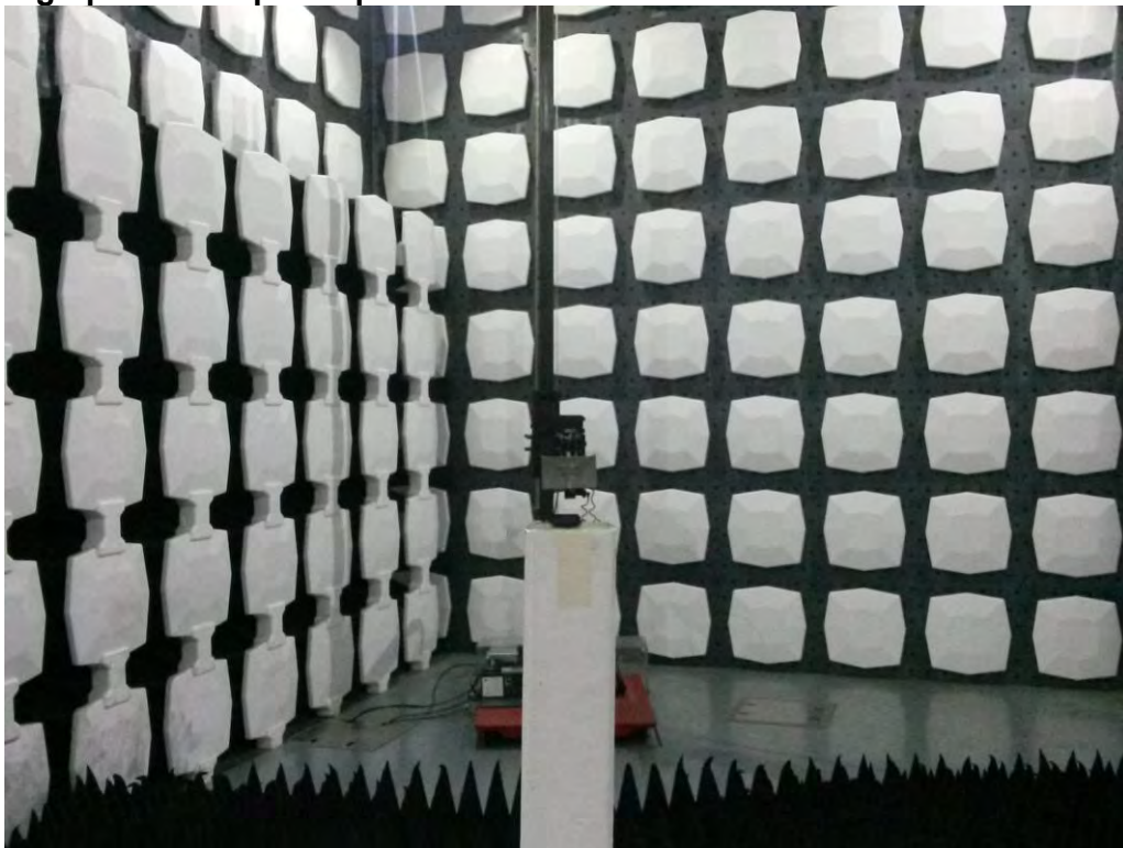
Photograph 4: Set-up for Spurious Emissions of 1 – 18GHz of IC
