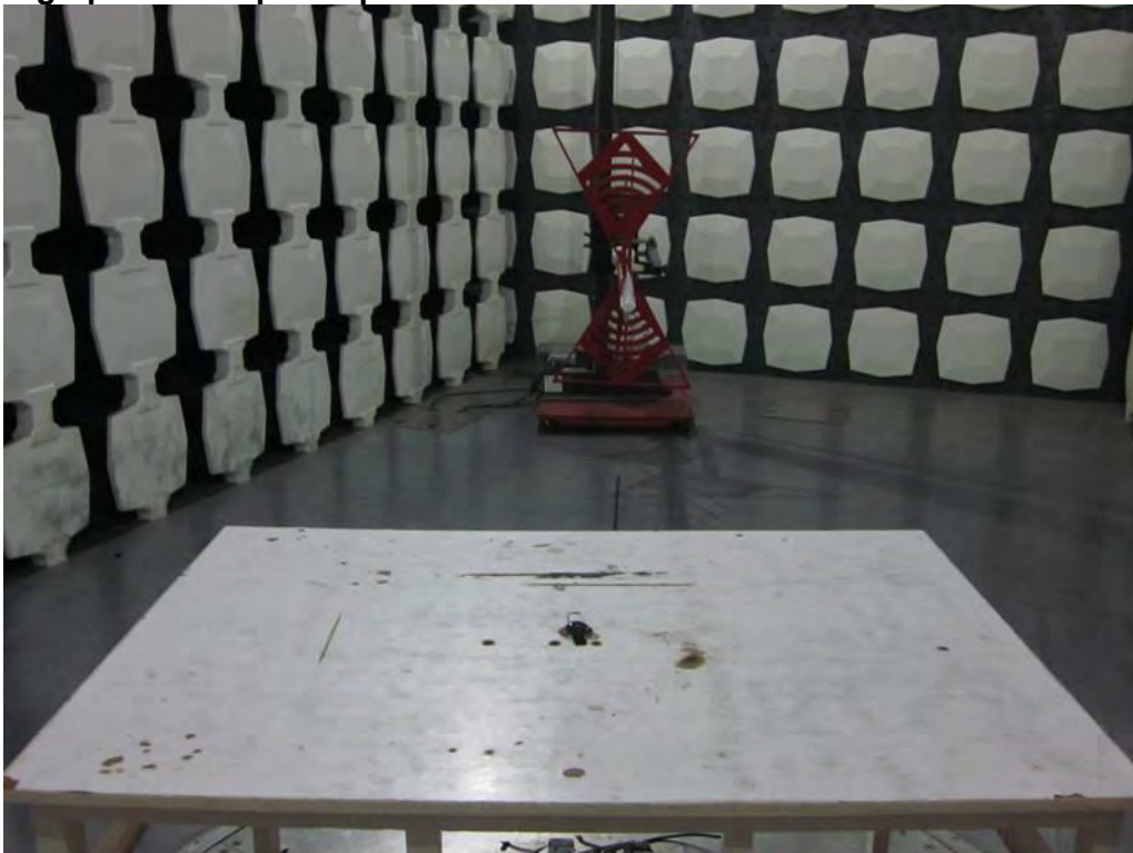
Photograph 2: Set-up for Spurious Emissions of 30MHz – 1GHz
