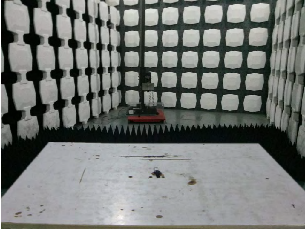
Photograph 4: Set-up for Spurious Emissions of 1 – 18GHz of IC
